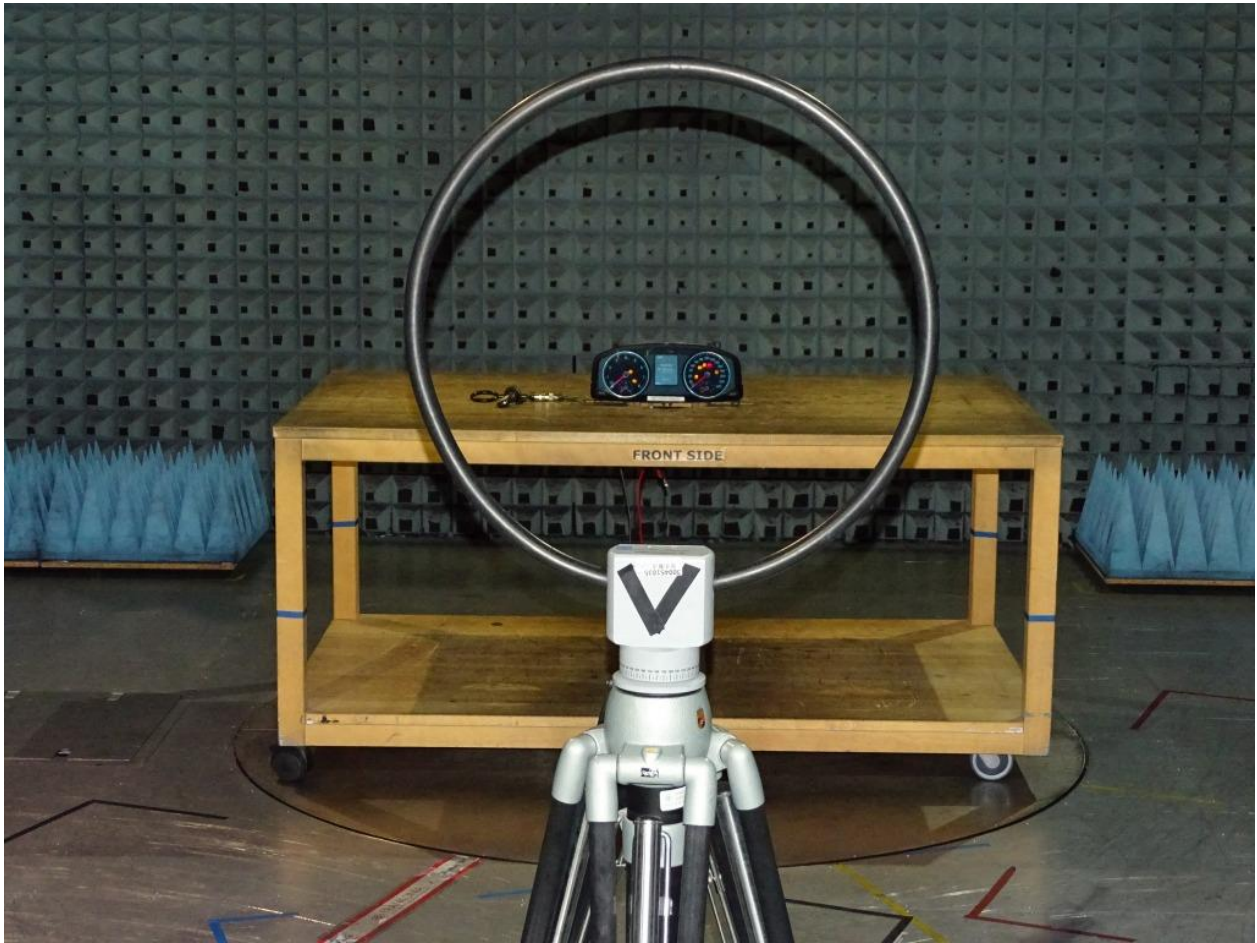
Photo 1: Test setup for radiated measurements (Enclosure, below 30 MHz, intentional radiator §15.209, ANSI C63.10)
