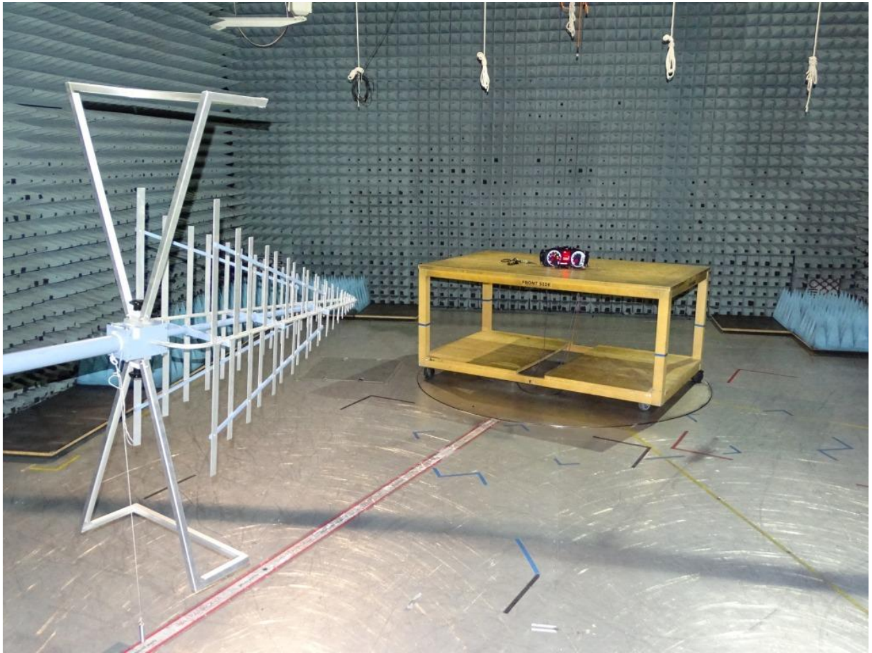
Photo 2: Test setup for radiated measurements (Enclosure, semi-anechoic chamber, 30 MHz to 1 GHz, intentional radiator §15.209, ANSI C63.10)
