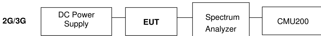
Fig. 2-1 Configuration of Tested System (Fixed Channel-Conducted)
