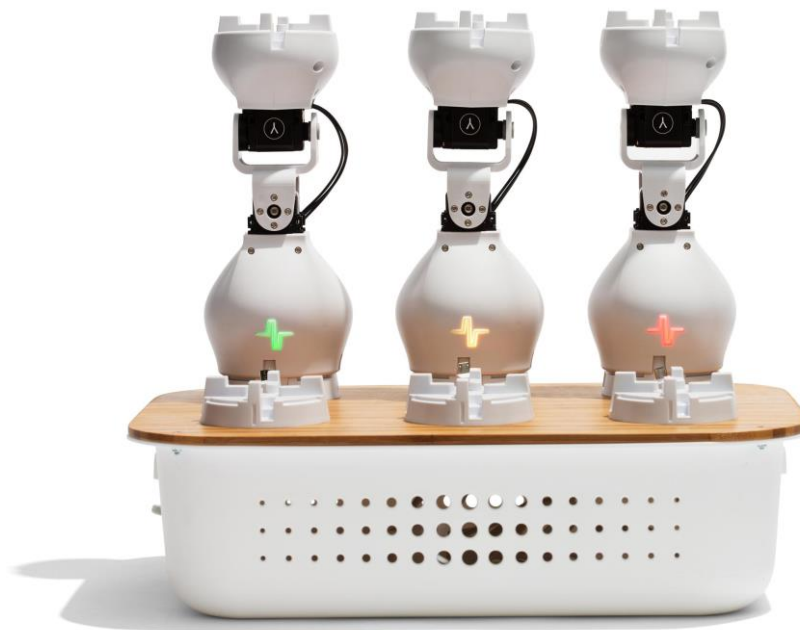
Figure 7 - Joint Modules being charged by using a charging station. Each module shows a different battery level. Where green depicts full battery, yellow is medium level, and red is low level.
