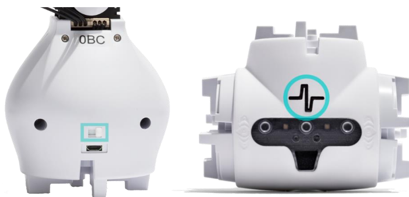
Figure 6 - Turn the switch left and right to turn the Joint module (left) on or off. For Fable Spin press on the Shape logo for 3 seconds to put in sleep mode.
