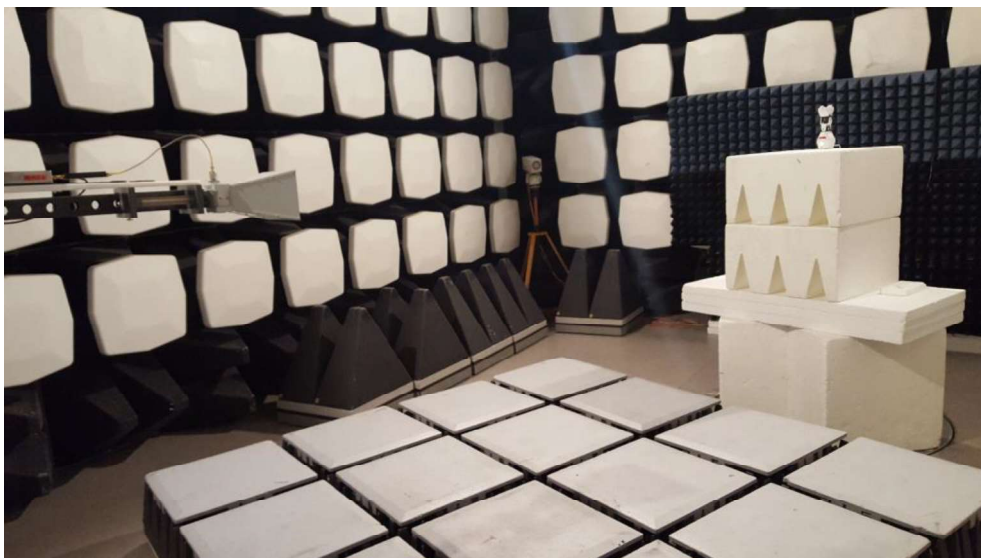
Photo 6 - Radiated emission test setup for 1 - 14 GHz.
