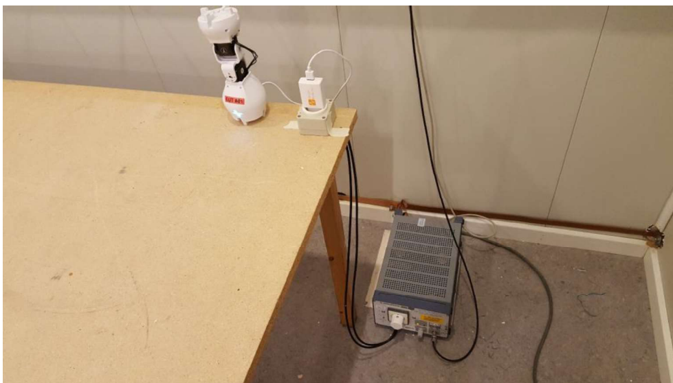
Photo 8. AC Conducted emission test set up.
