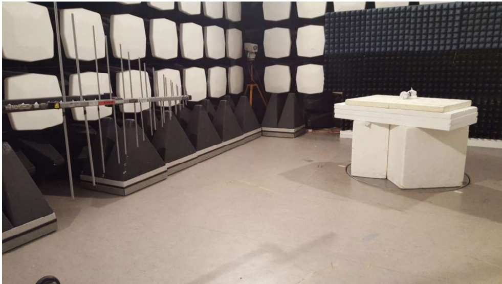
Photo 5 - Radiated emission test setup for 200 - 1000 MHz.
