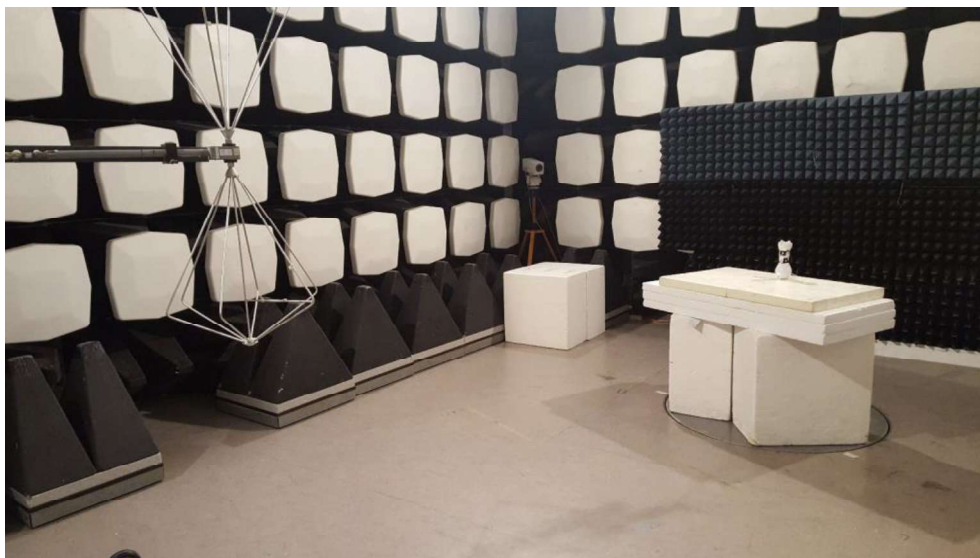
Photo 4 - Radiated emission test setup for 30 - 200 MHz.
