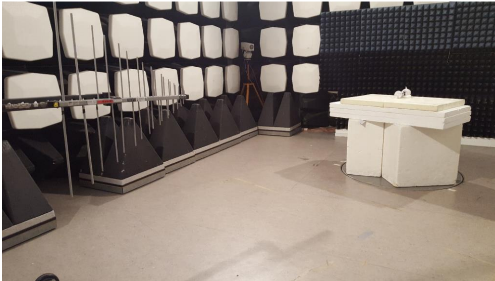
Photo 5 - Radiated emission test setup for 200 - 1000 MHz.
