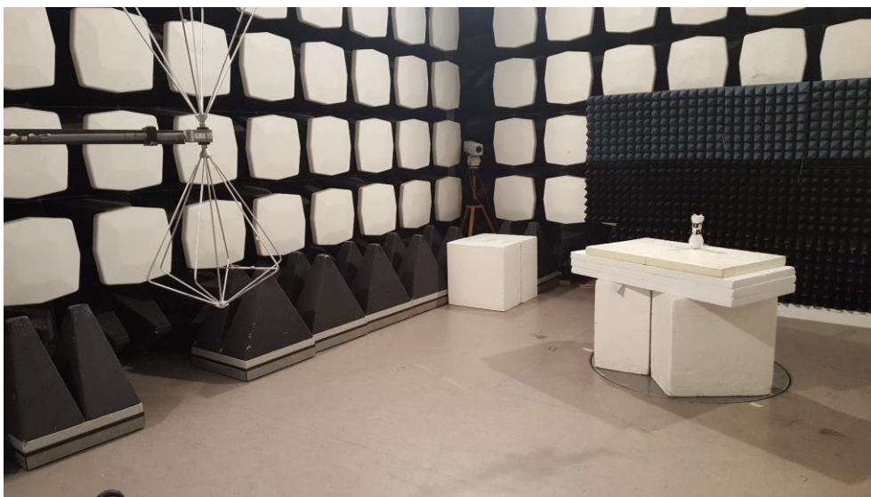
Photo 4 - Radiated emission test setup for 30 - 200 MHz.
