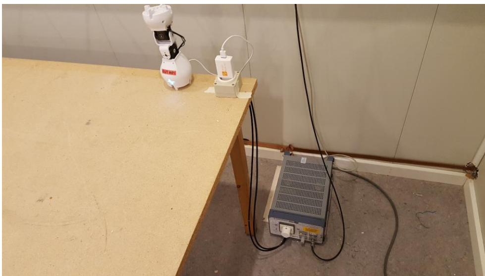
Photo 8. AC Conducted emission test set up.
