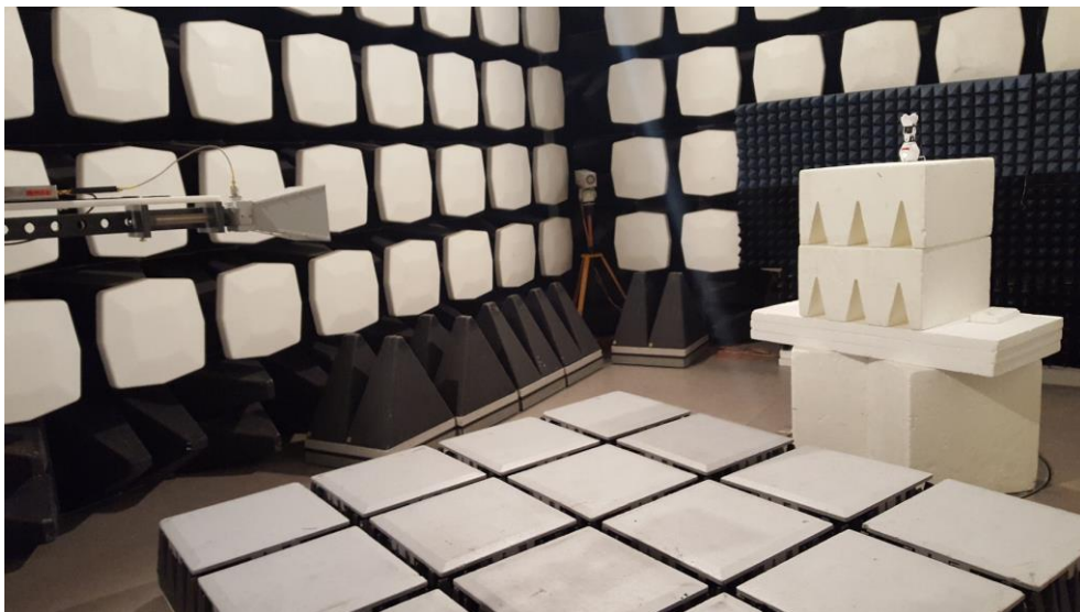
Photo 6 - Radiated emission test setup for 1 - 14 GHz.
