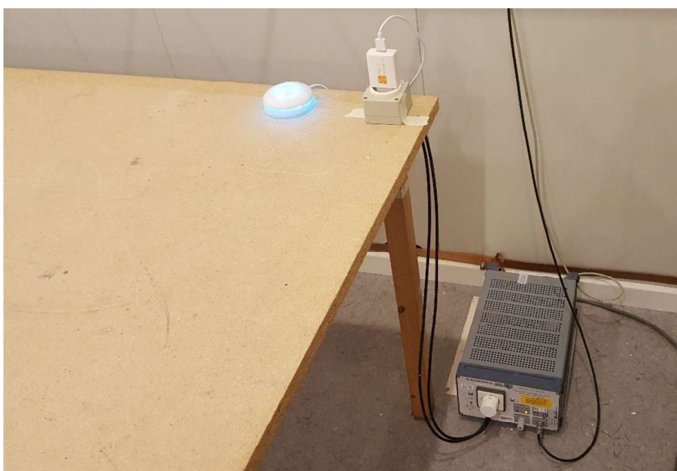
Photo 11. AC Conducted emission test set up. Powered by AC/DC adaptor
