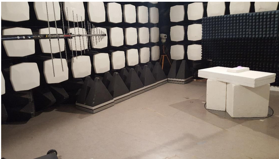
Photo 4 - Radiated emission test setup for 200 - 1000 MHz.
