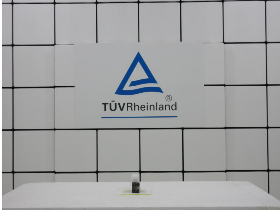
Photograph 1: Test Setup for Spurious Emissions (Front View 1)
