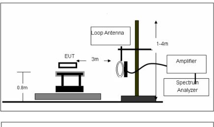
6.1 Block Diagram of Test Setup
