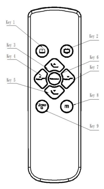
Key 1: Short press button 1, and the fader will run to a fixed position (Book mode) to stop; long press button 1, after 3 seconds, the current position will be memorized (overwrite the previous memory), the backlight will flash 3 times quickly, and the control box will beep
