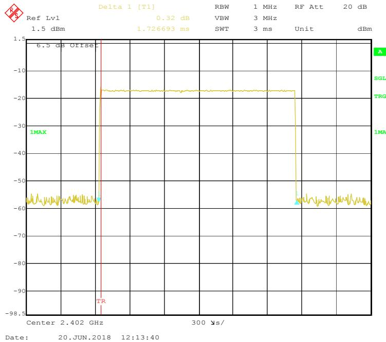
**EDR (8DPSK): Pulse time, Middle Channel, 3DH3**
