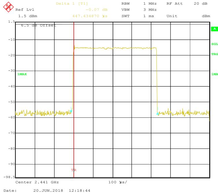
**EDR ( $\pi/4$ -DQPSK):Pulse time, High Channel, 2DH1**
