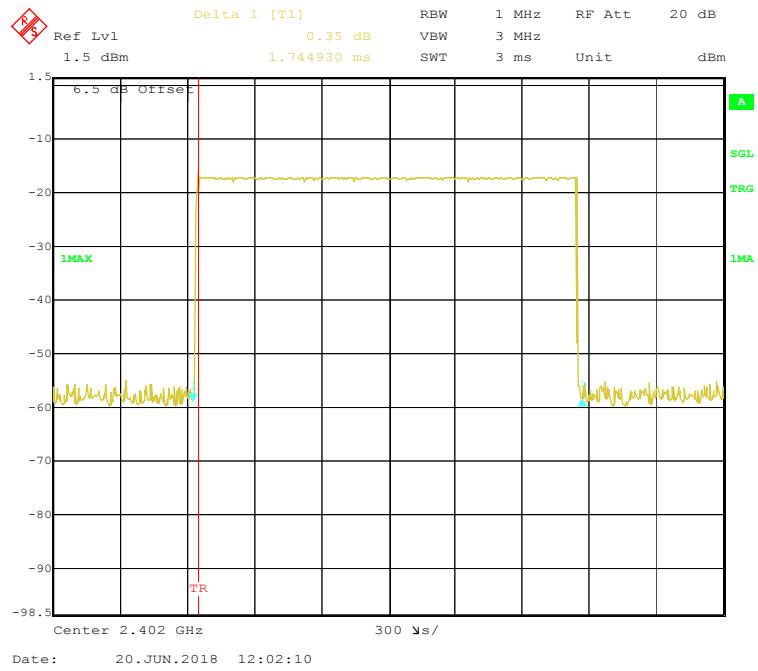
**EDR ( $\pi/4$ -DQPSK):Pulse time, Middle Channel, 2DH3**
