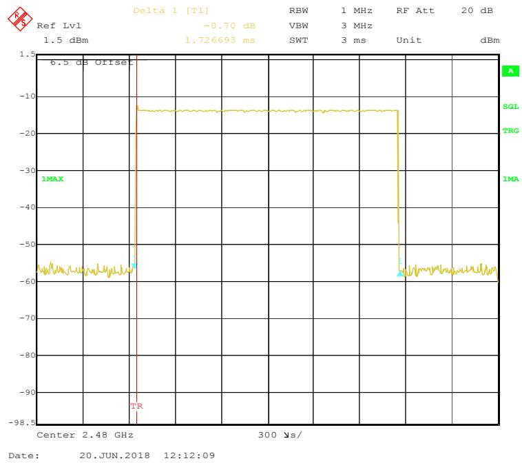
**EDR (8DPSK): Pulse time, Low Channel, 3DH5**
