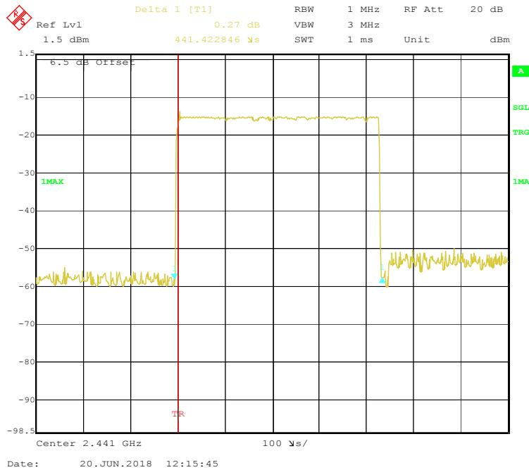
**BDR (GFSK): Pulse time, High Channel, DH1**
