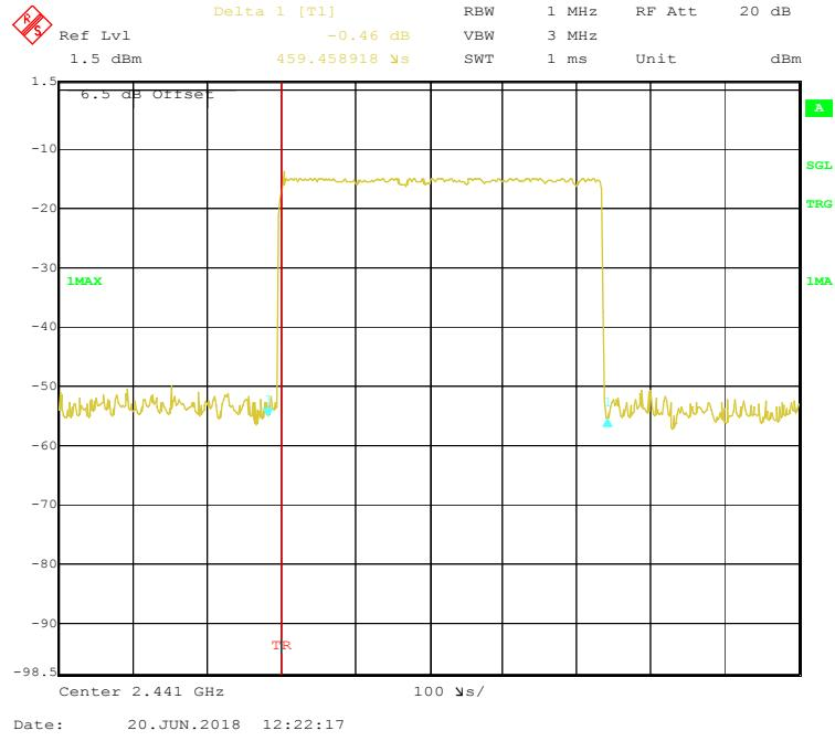
**EDR (8DPSK): Pulse time, High Channel, 3DH1**
