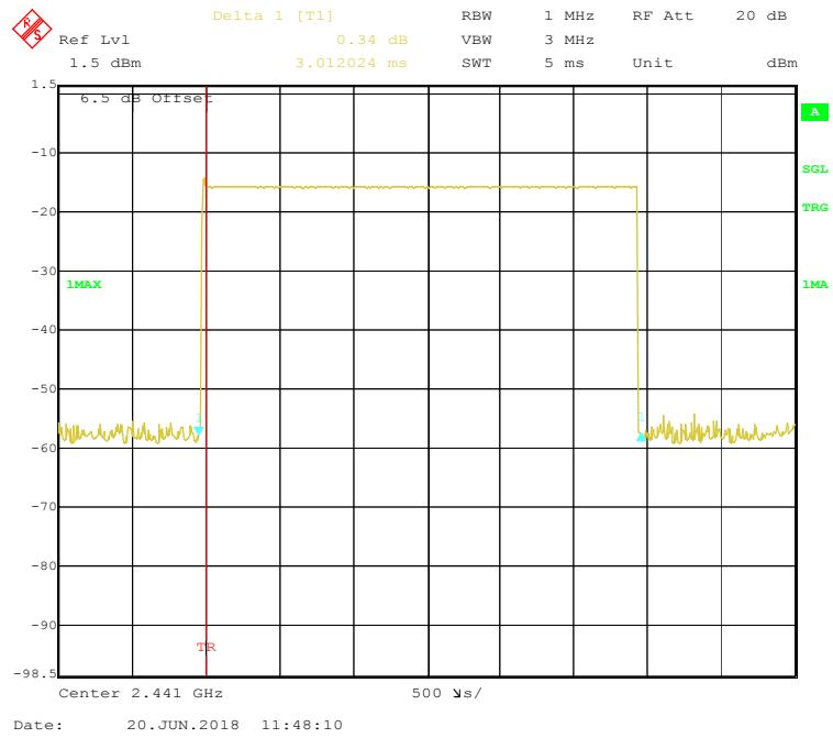
**EDR ( $\pi/4$ -DQPSK):Pulse time, High Channel, 2DH5**
