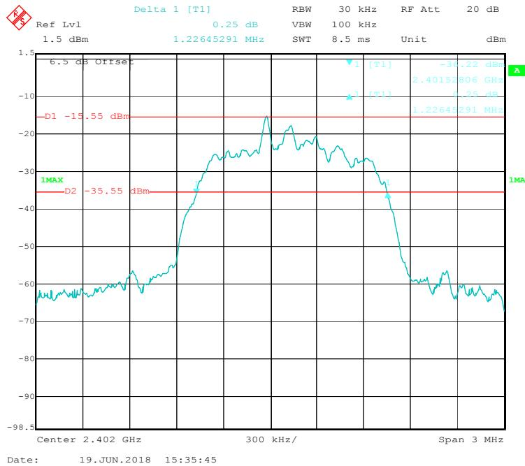
**EDR (8DPSK): Middle Channel**
