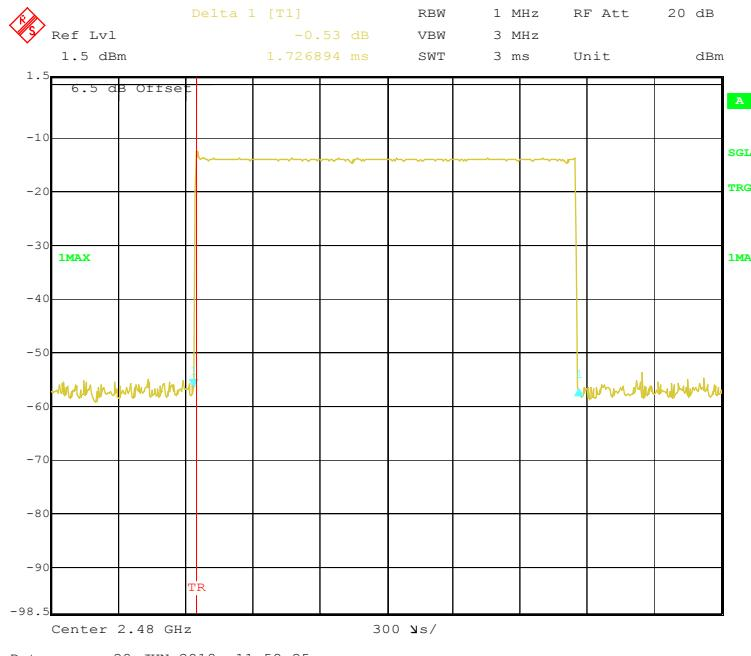
**BDR (GFSK): Pulse time, Low Channel, DH5**
