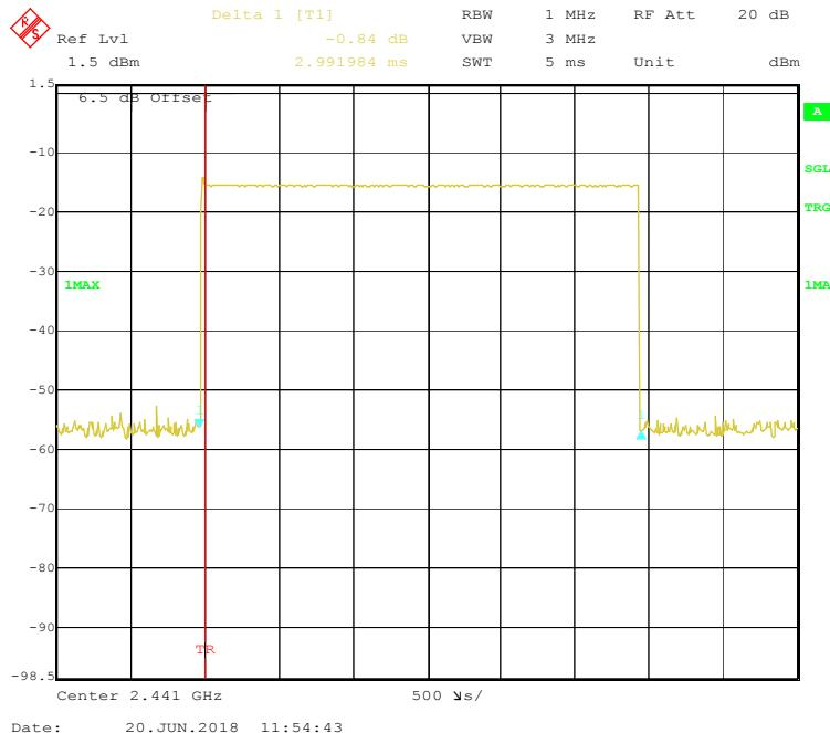
**BDR (GFSK): Pulse time, High Channel, DH5**
