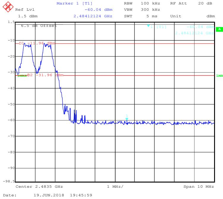
**EDR (8DPSK): Left Side- Hopping**
