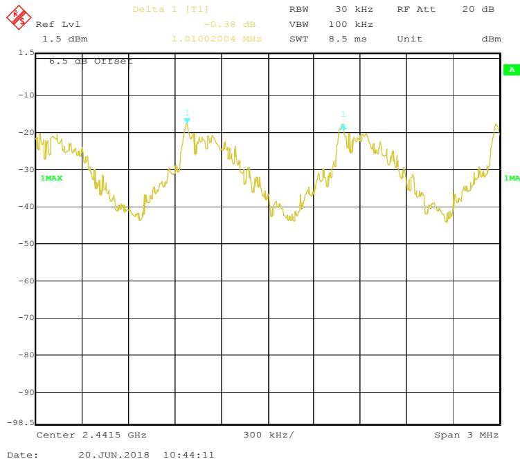
**EDR ( $\pi/4$ -DQPSK): High Channel**
