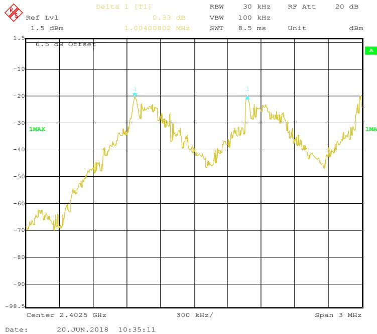
**EDR (8DPSK): Middle Channel**
