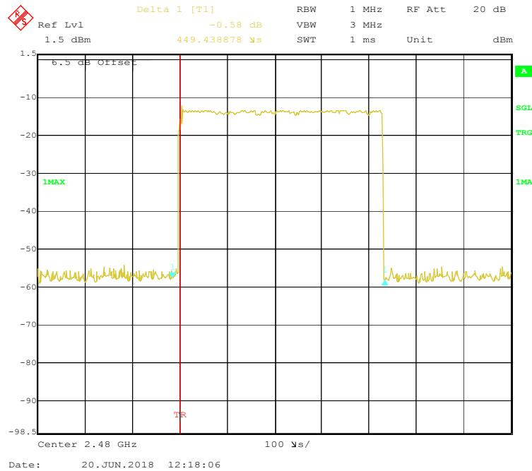
**EDR ( $\pi/4$ -DQPSK):Pulse time, Low Channel, 2DH3**
