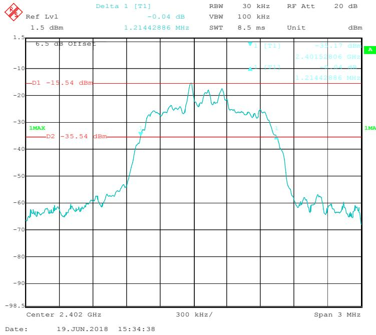
**EDR( $\pi/4$ -DQPSK): Middle Channel**
