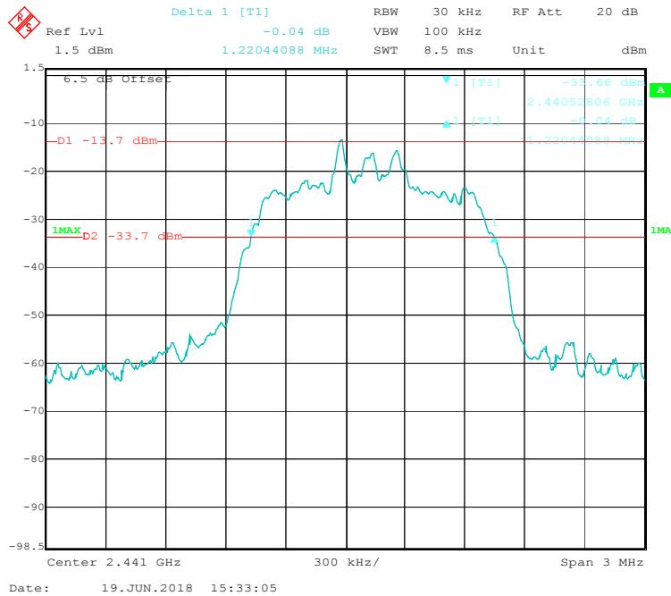
**EDR ( $\pi/4$ -DQPSK): High Channel**
