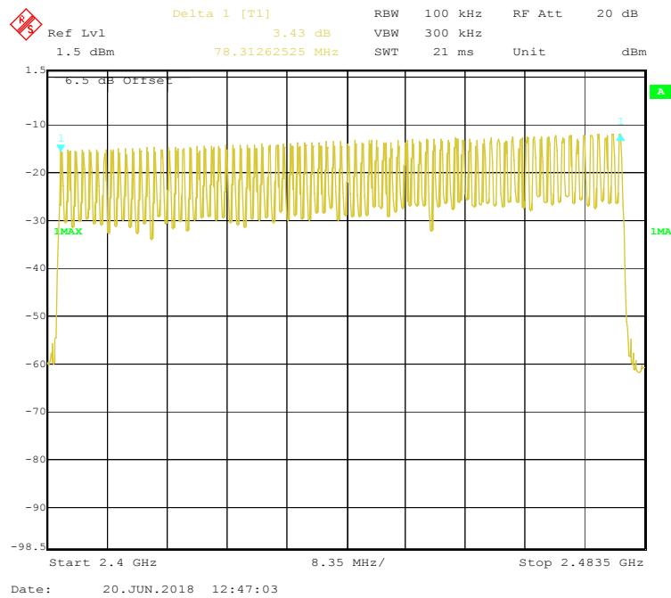
**EDR ( $\pi/4$ -DQPSK): Number of Hopping Channels**
