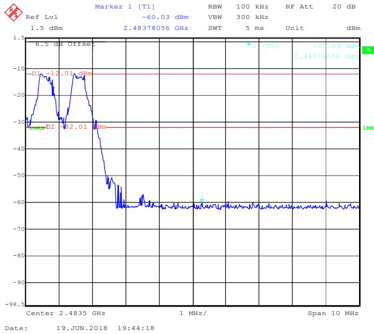
**EDR ( $\pi/4$ -DQPSK): Left Side- Hopping**
