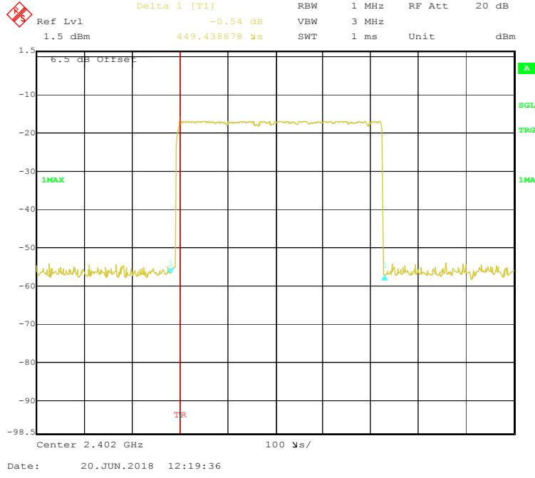
**EDR ( $\pi/4$ -DQPSK):Pulse time, Middle Channel, 2DH1**
