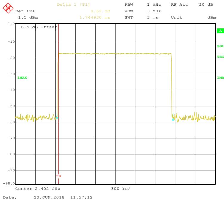
**BDR (GFSK): Pulse time, Middle Channel, DH3**
