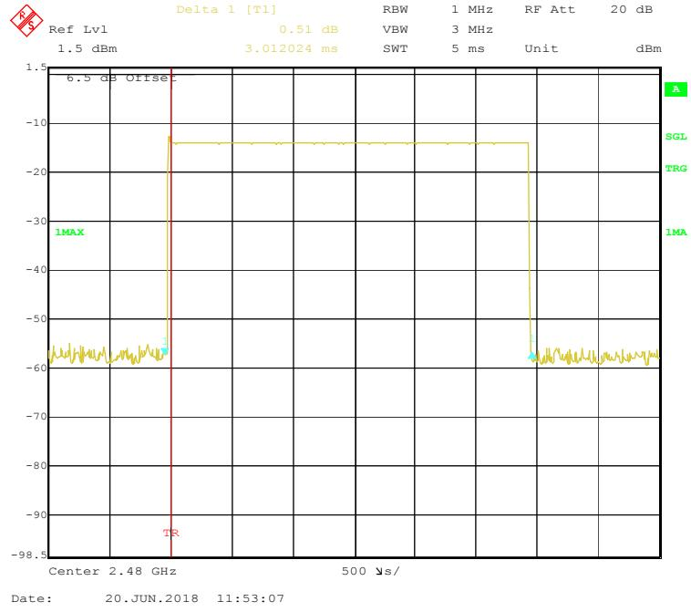
**EDR (8DPSK): Pulse time, Low Channel, 3DH1**
