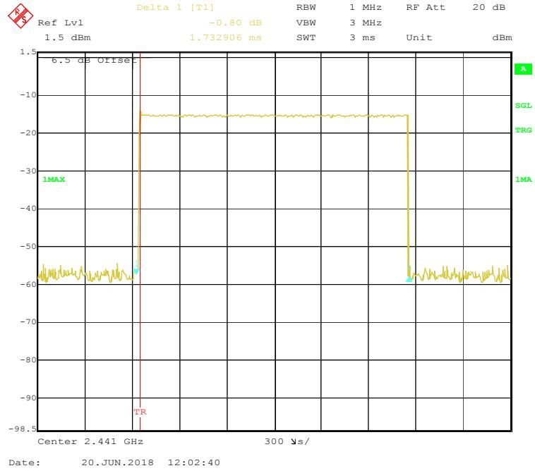
**EDR ( $\pi/4$ -DQPSK):Pulse time, High Channel, 2DH3**
