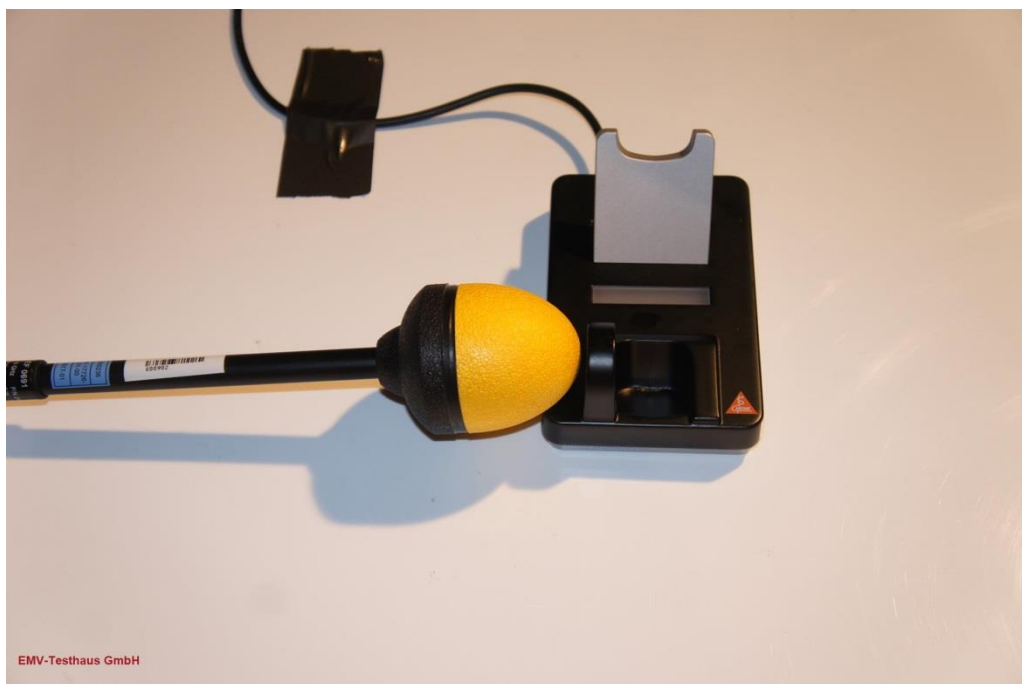
Picture 9: Setup of electric field test for standby mode
