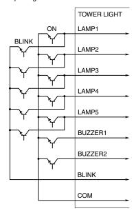
Note: If "On" and "Blink" are set simultaneously for a single lamp, "Blink" is disabled.
