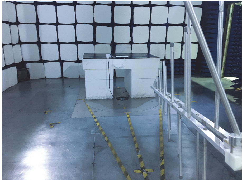
Radiation Emission Test Setup (30MHz to 1GHz)
