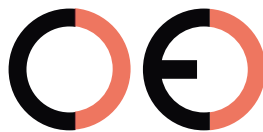
False CE Mark (too far)
