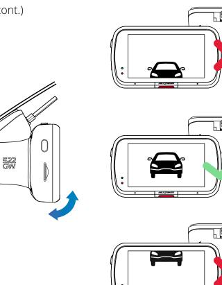
9 Adjusting the Dash Cam With the mount attached to the windscreen, ensure that objects on the Dash Cam display are level and adjust as required. Ensure that the road ahead is at the centre of the image, in the central third of the display. If too much of the sky is visible it may risk underexposing details on the road; ensure that the road ahead is clearly visible on the Dash Cam display. Do NOT attempt to adjust the Dash Cam while driving.
