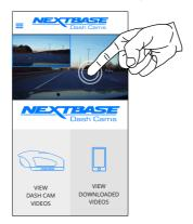
Tapping the Front Facing Camera view will make the Live view full screen, rotated to fill your screen. To exit this view, simply tap the screen again to reveal the back arrow (top left).
