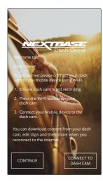
Tap the CONNECT TO DASH CAM Button and Nextbase Cam Viewer will then open your Settings screen for your mobile device.
