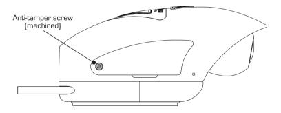
Carefully insert the supplied rubber dust caps, covering the heads of the anti-tampers screws.
