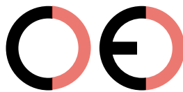
False CE Mark (too far)
