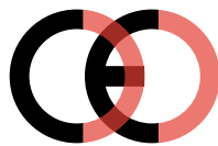
False CE Mark (too close)
