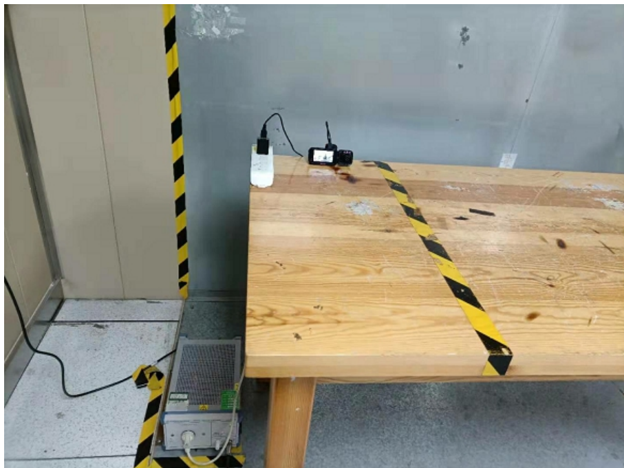
Conducted emission Test Setup
