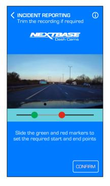
To trim the video use the GREEN button to select the new start point and the RED button to set the new end point of the recording.
