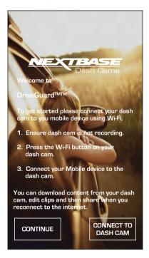
Tap the CONNECT TO DASH CAM button and Nextbase DriveGuard™ will then open the Settings screen for your mobile device.
