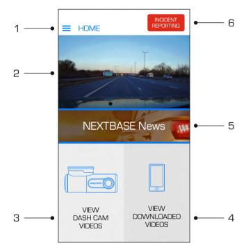
From within the Main screen you can select Live View, view recordings stored on your Dash Cam or recordings that have previously been downloaded to your mobile device. You can also access the Nextbase DriveGuard™ Menu options.
