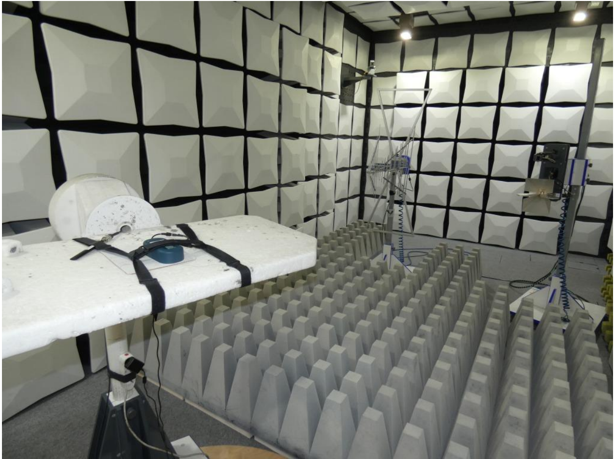
Photo 3: Test setup for radiated measurements (Enclosure, fully-anechoic chamber)
