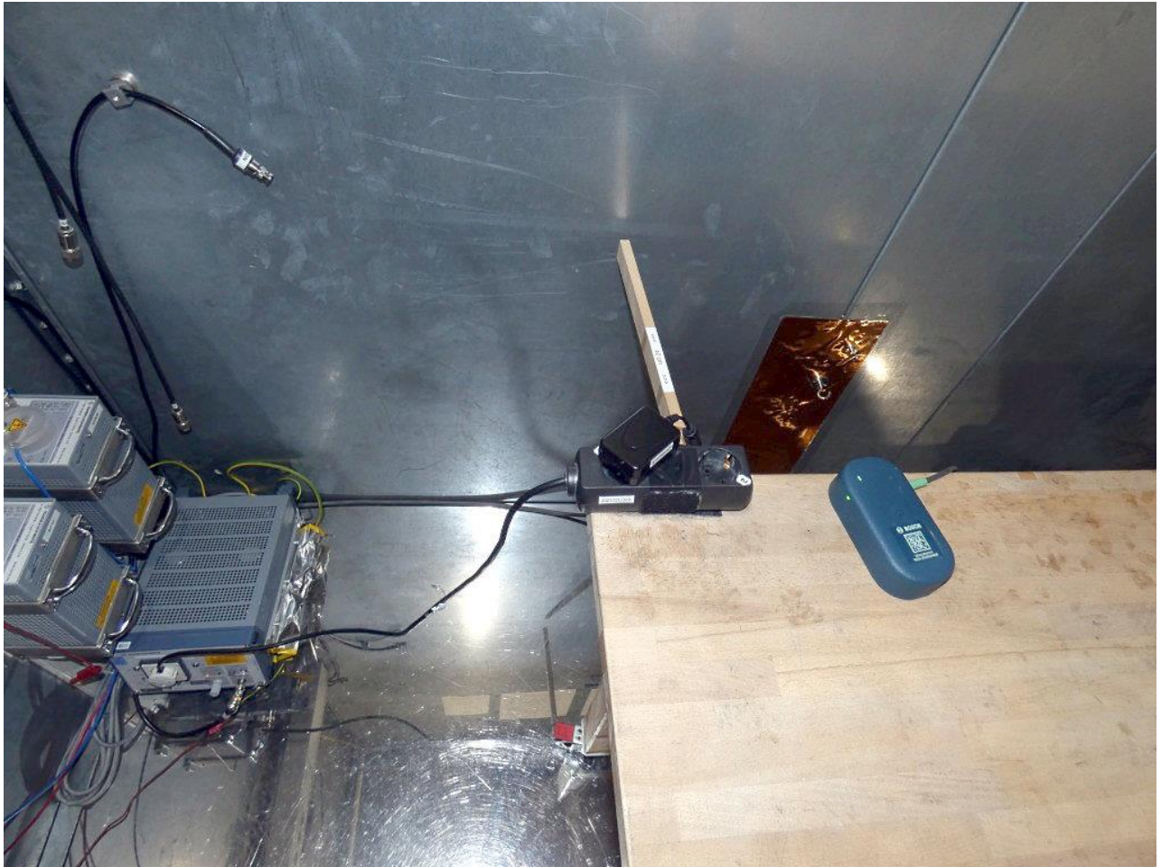
Photo 4: Test setup for conducted measurements (AC Port (power line), EUT supplied by AC/DC adapter, intentional / unintentional radiator §15, ANSI C63.10/4)
