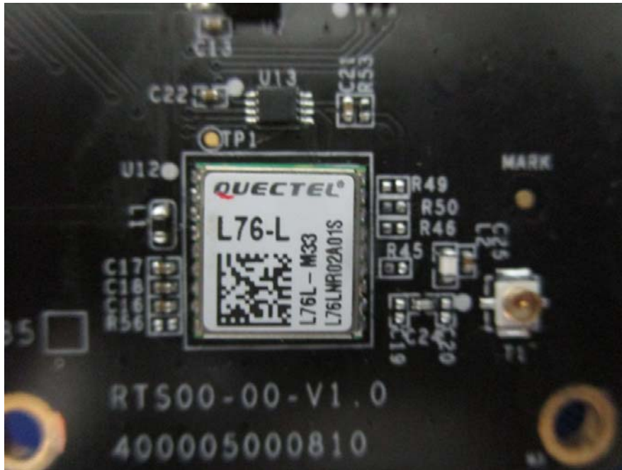
EUT – GPS module View
