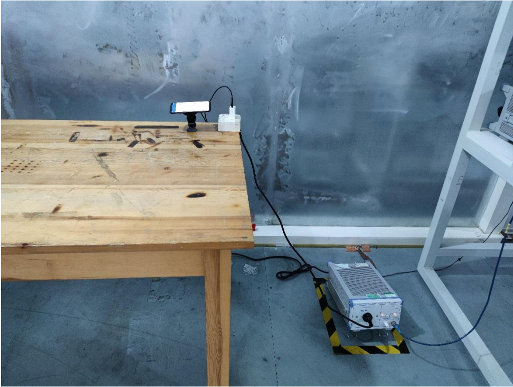
Conducted Emission-AC adapter charge mode
