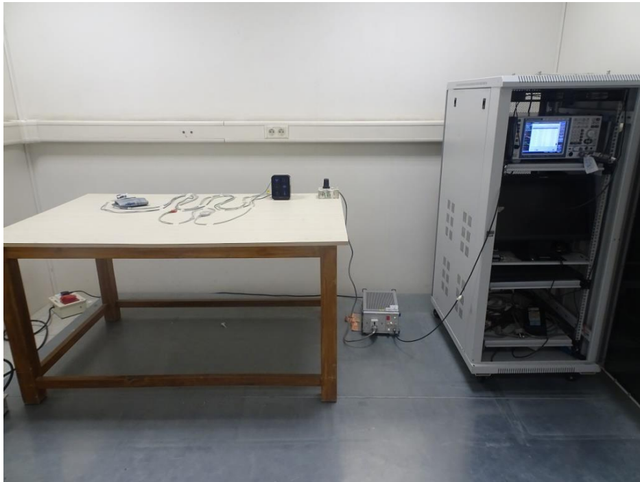
Test setup Conducted Emission Test on A.C. Power Line
