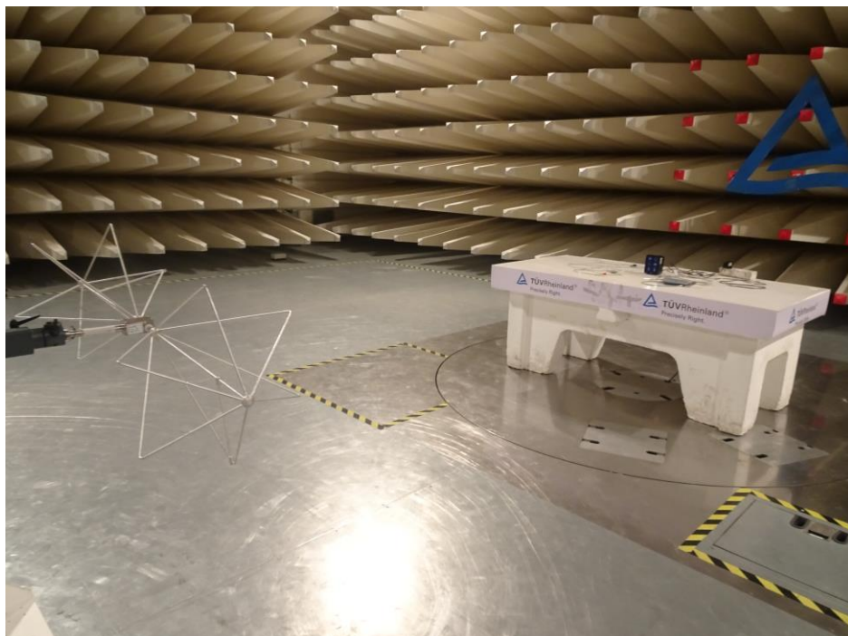
Test setup Frequency Range 30MHz-200MHz Biconical Antenna
