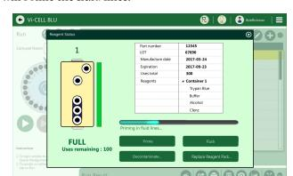
**5** The instrument will Prime the fluid lines.
