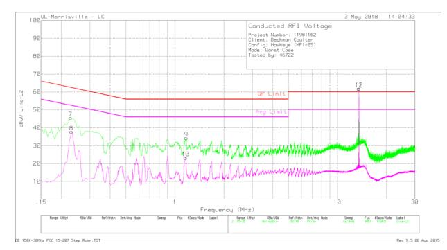
Range 2: Line-L2 .15 - 30MHz Meter Corrected Frequency Cbl/Limiter Margin Margin Reading Reading LISN VCF (dB) **QP** Limit Marker Det Avg Limit (MHz) (dB) (dB) (dB) (dBuV) dBuV 7 .228 35.56 Ρk .1 9.9 45.56 62.52 -16.96 -8 .231 27.72 9.9 37.72 52.41 -14.69 Av .1 \_ \_ 9 1.176 24.41 Ρk 0 9.9 34.31 56 -21.69 --10 1.164 13.31 Av 0 9.9 23.21 --46 -22.79 13.56<sup>1</sup> 11 51.78 Ρk .1 10.1 61.98 ----13.56<sup>1</sup> 10.1 12 51.56 .1 61.76 ---Av -
