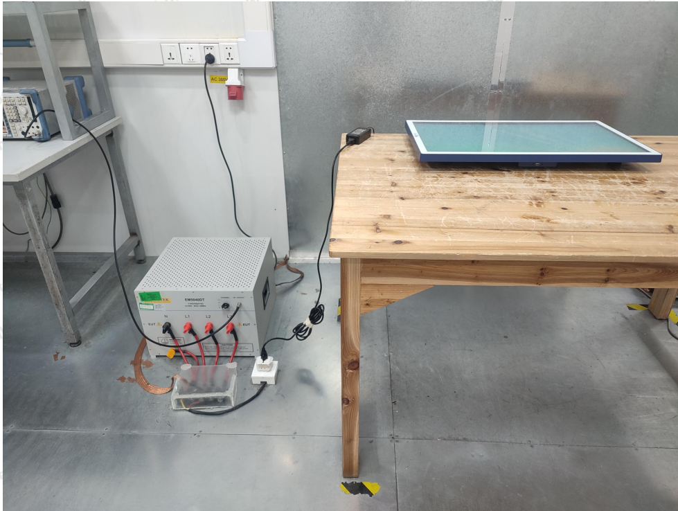
Photo of Conducted Emission Measurement
