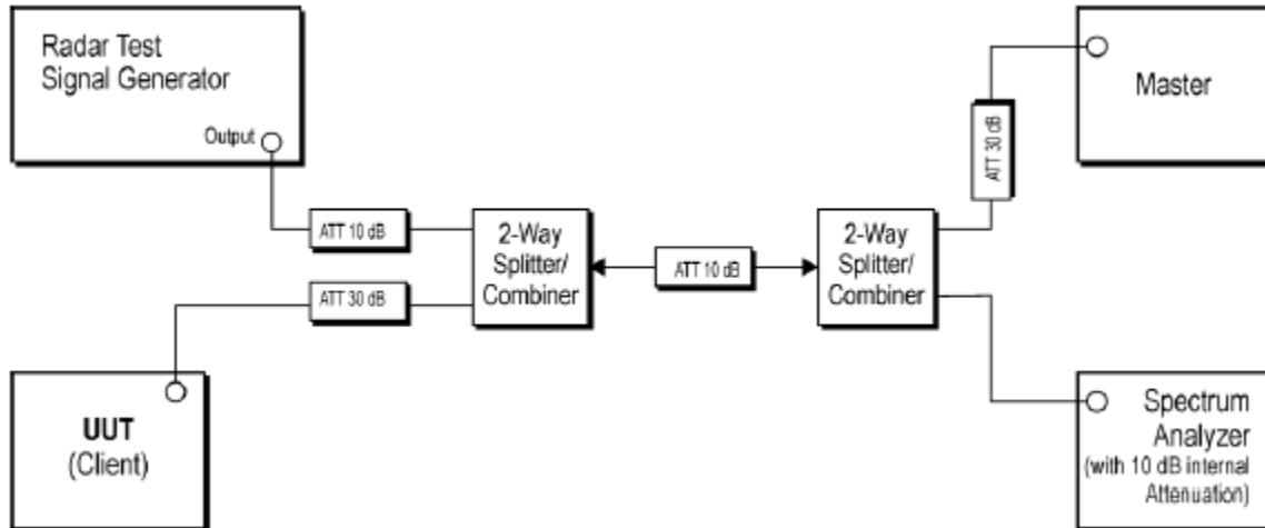
2. The radar test signal level was set at the Master Device – Radar Detection Device according to the appropriate DFS Detection Threshold.
