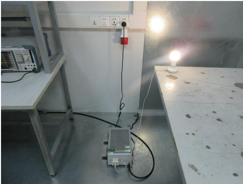
Photo of Conducted Emission Measurement
