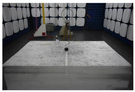
3. Radiated emission (9KHz-30MHz)
