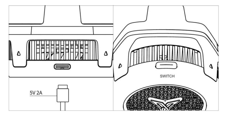
1. First to use: The default mode is the Smart Frequency Conversion mode. Notice: 5V 2A or higher charger output is required.
