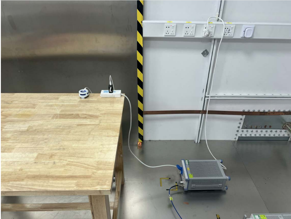
AC Power Line Conducted Emission
