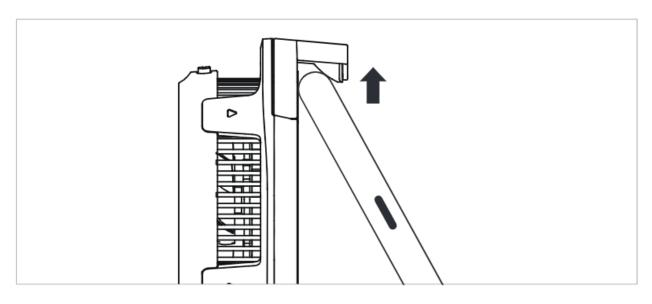
手持手机,抵住上槽后向上推 Hold mobile phone and push up against upper pull hook
