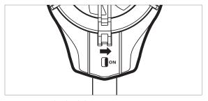
Connect power supply and toggle device ON. 连接电源,拨动开关至ON
