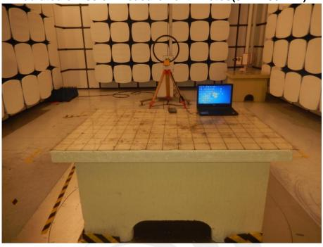
Radiated emission Measurement Photos(30MHz-1000MHz)
