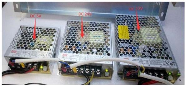
The red switch can be used to adjust the input of the power supply, and to the left is 100-120v ac input, to the right is 200-240v ac input. As the picture follows:
