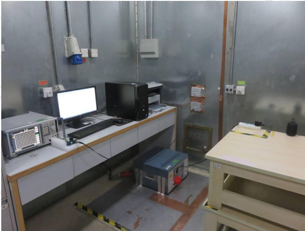
FCC RADIATED EMISSION TEST SETUP
