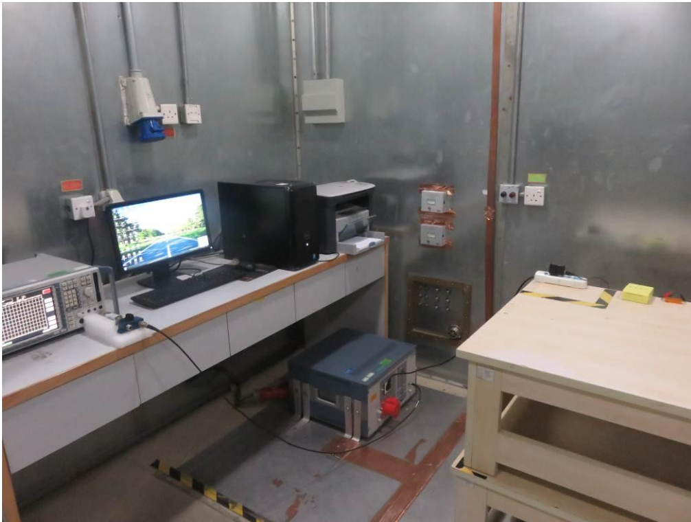
FCC RADIATED EMISSION TEST SETUP
