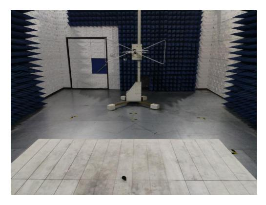
RADIATED EMISSION TEST SETUP ABOVE 1GHZ
