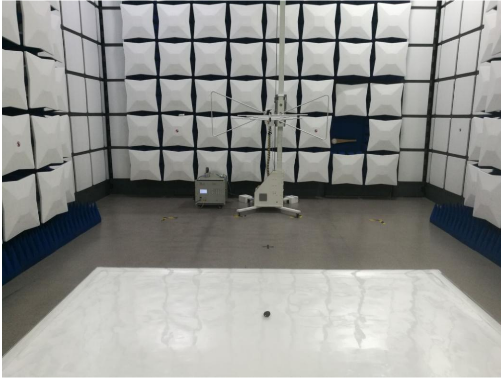
FCC RADIATED EMISSION TEST SETUP
