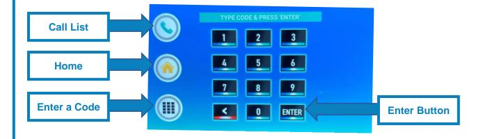
The Code will activate Relay 1 (the gate should open).
