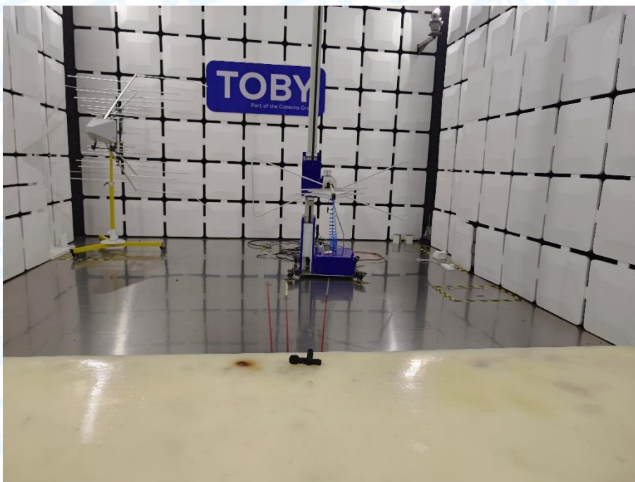
Photo of Setup for Radiated Emission (30MHz~1GHz)
