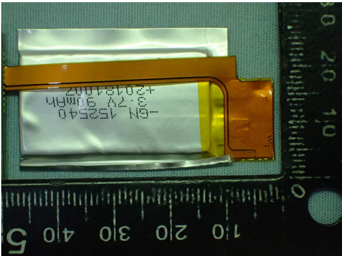
Figure 14 Internal View (Battery)
