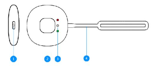
Charge Spot: Attach power cord to it to charge the alarm.
