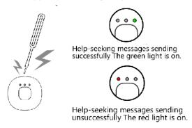
Press the button to give an alarm: when you are in emergency circumstances, you can press the button for two times. If the green light is on, it means you have called the police successfully. If the red light flashes, it means you haven't called the successfully.
