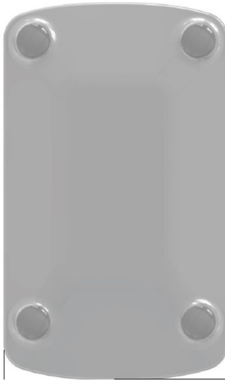
Fig. 4. Back of the recorder with electrodes
