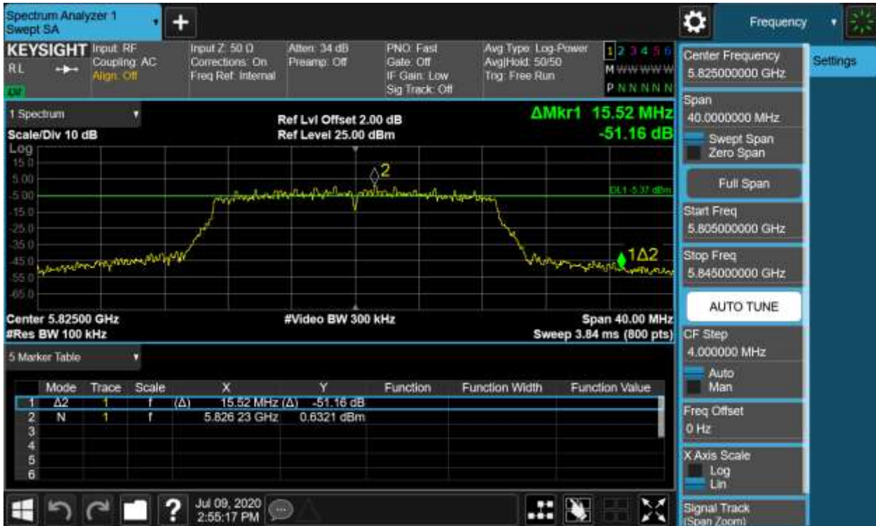
Figure 37: 6dB Bandwidth, 802.11ac(VHT20), 5825MHz
