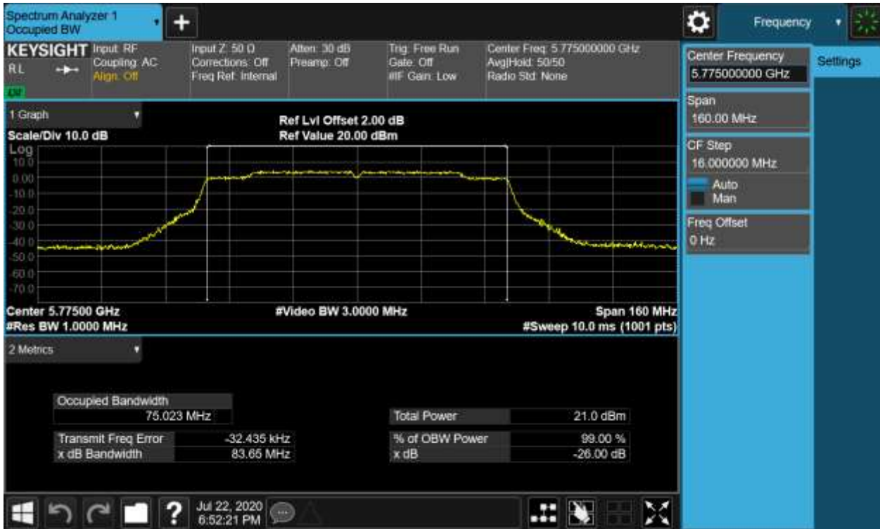
Figure 28: 26dB Bandwidth and 99% Bandwidth, 802.11ac(VHT80), 5775MHz
