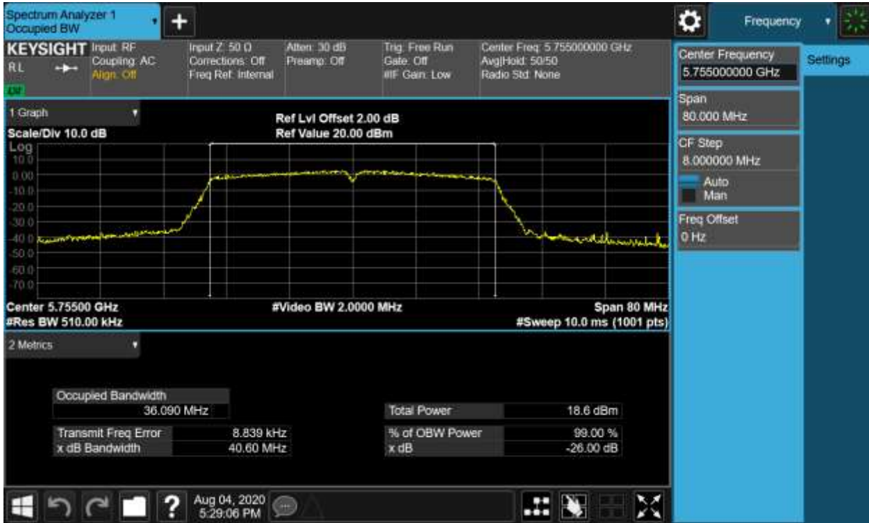
Figure 26: 26dB Bandwidth and 99% Bandwidth, 802.11ac(VHT40), 5755MHz
