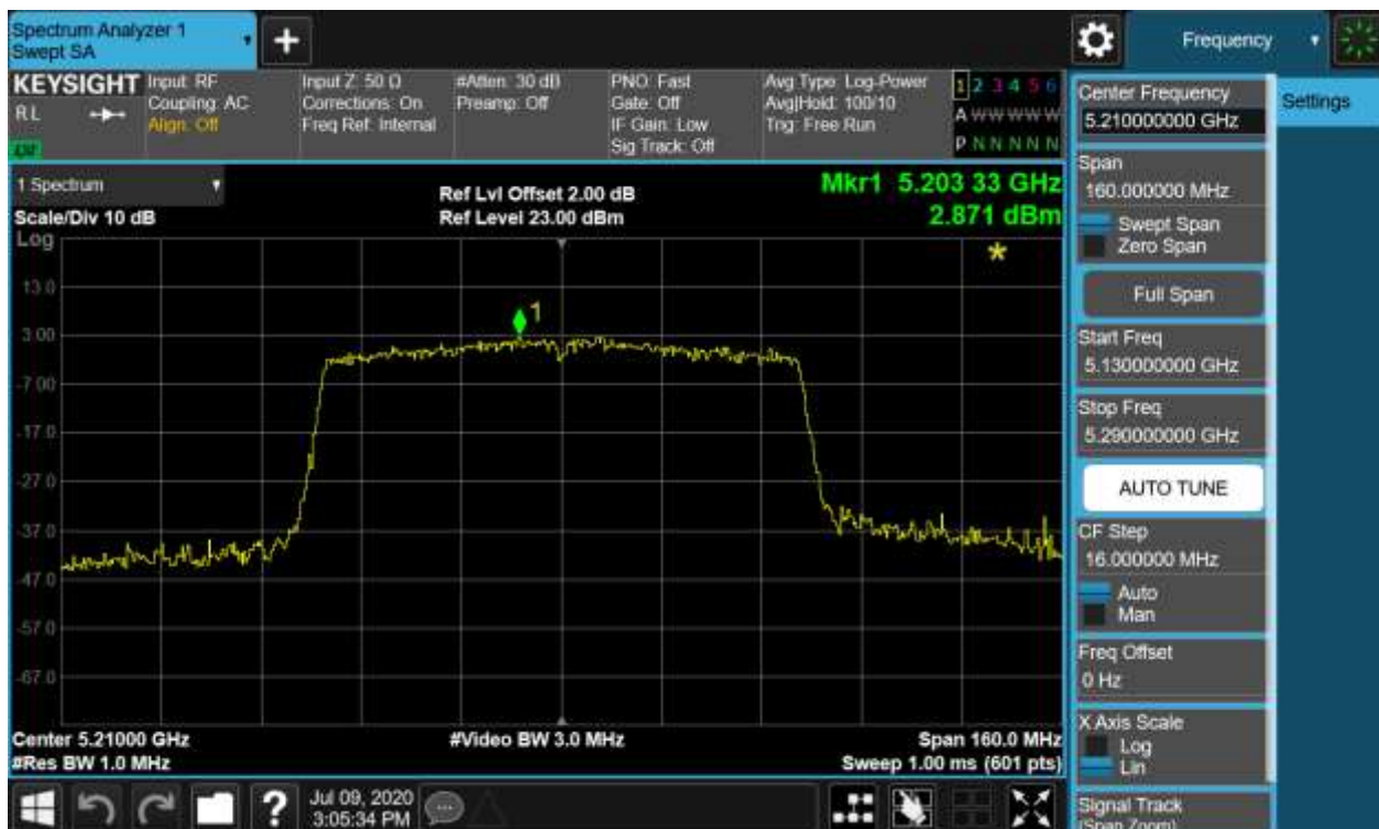
Figure 56: Power Spectral Density, 802.11ac(VHT80), 5210MHz
