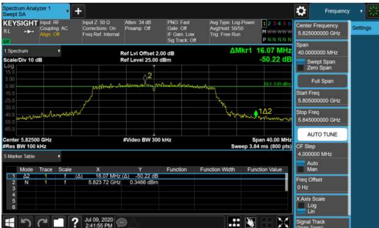
Figure 34: 6dB Bandwidth, 802.11n(HT20), 5825MHz
