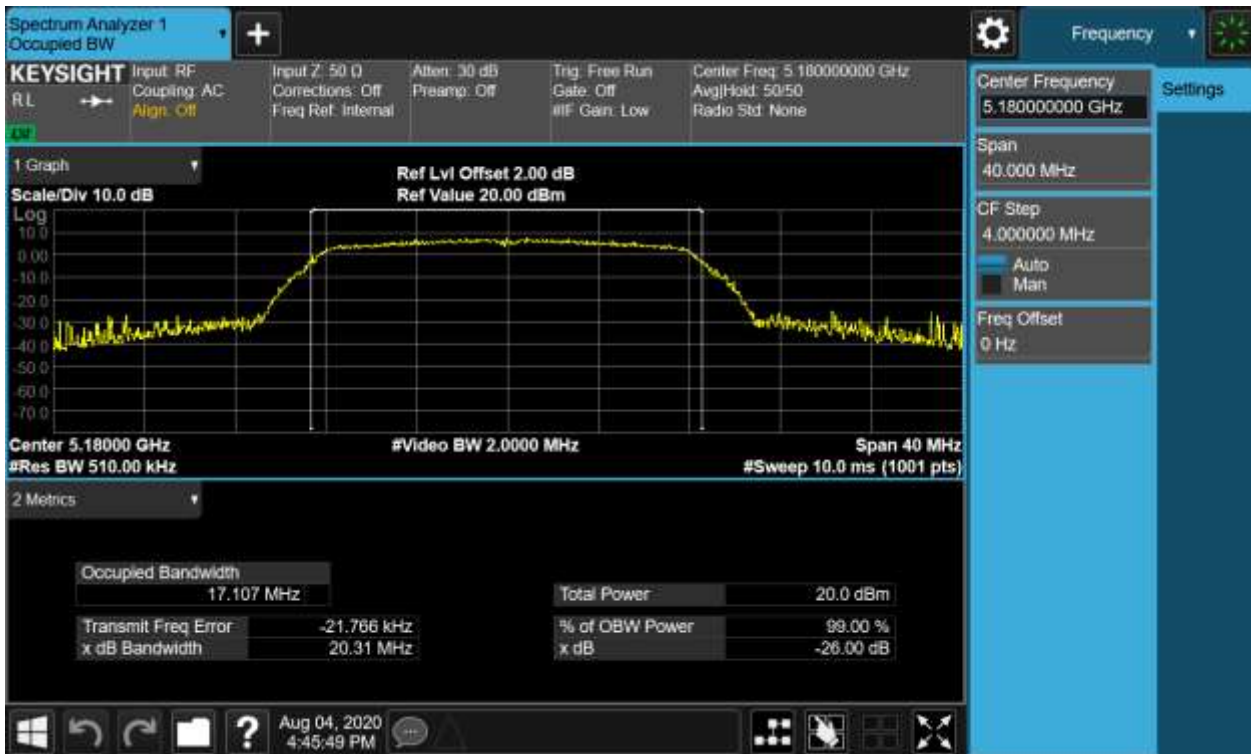
Figure 1: 26dB Bandwidth and 99% Bandwidth, 802.11a, 5180MHz
