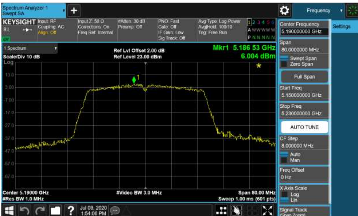
Figure 54: Power Spectral Density, 802.11ac(VHT40), 5190MHz
