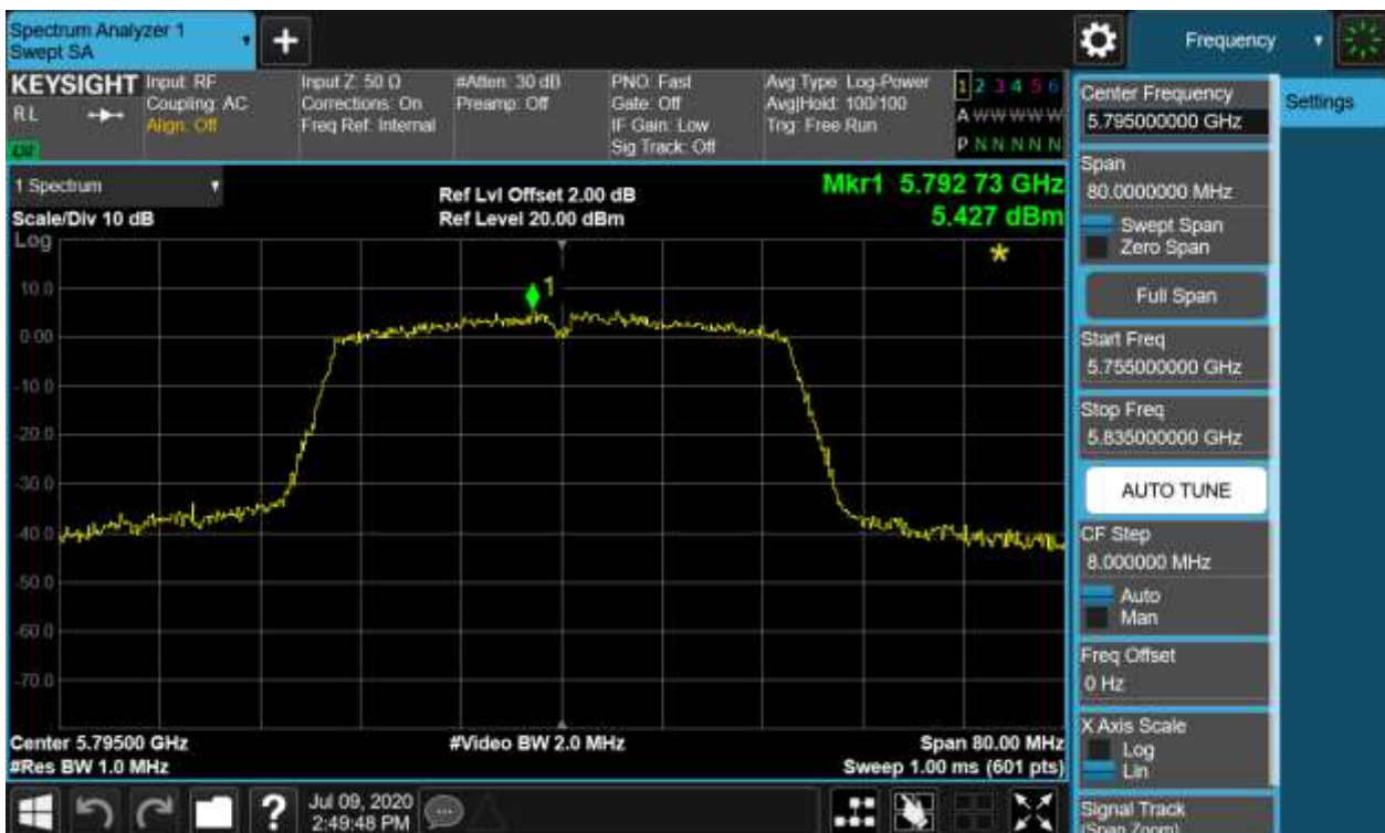
Figure 67: Power Spectral Density, 802.11n(HT40), 5795MHz
