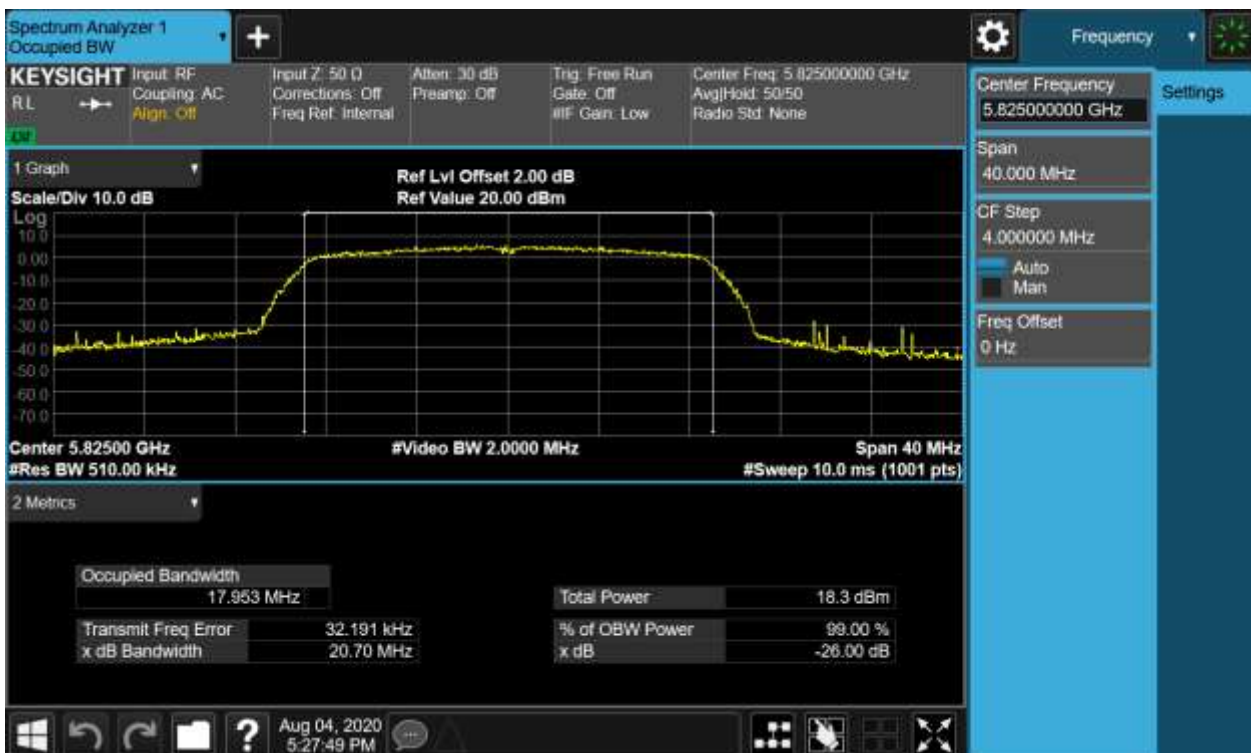
Figure 23: 26dB Bandwidth and 99% Bandwidth, 802.11ac(VHT20), 5825MHz
