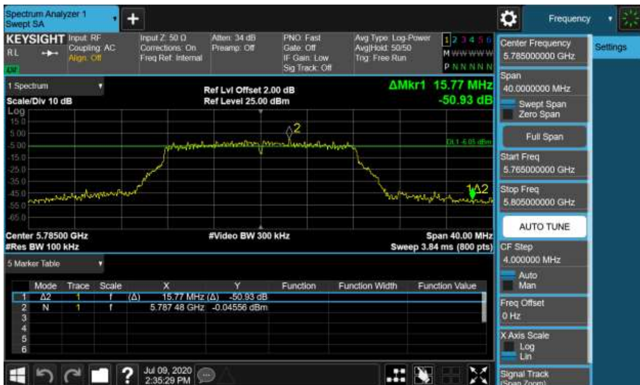
Figure 30: 6dB Bandwidth, 802.11a, 5785MHz
