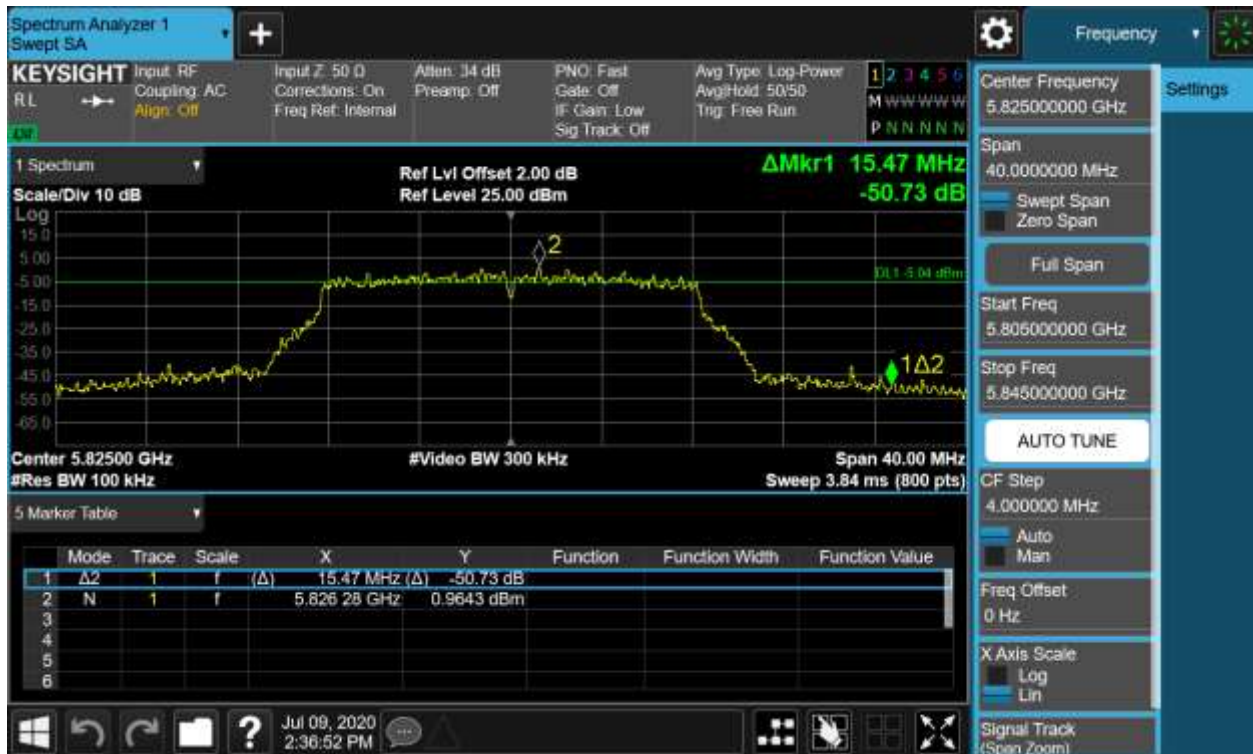
Figure 31: 6dB Bandwidth, 802.11a, 5825MHz
