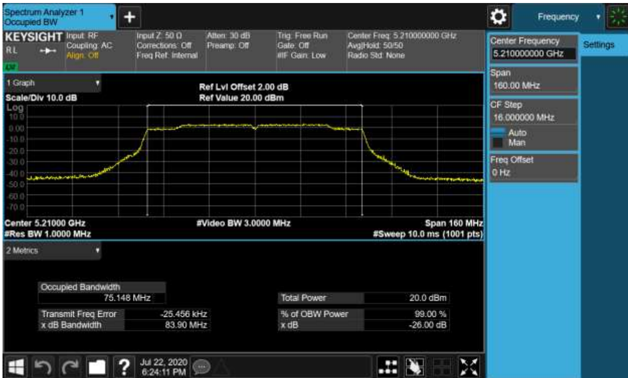
Figure 14: 26dB Bandwidth and 99% Bandwidth, 802.11ac(VHT80), 5210MHz
