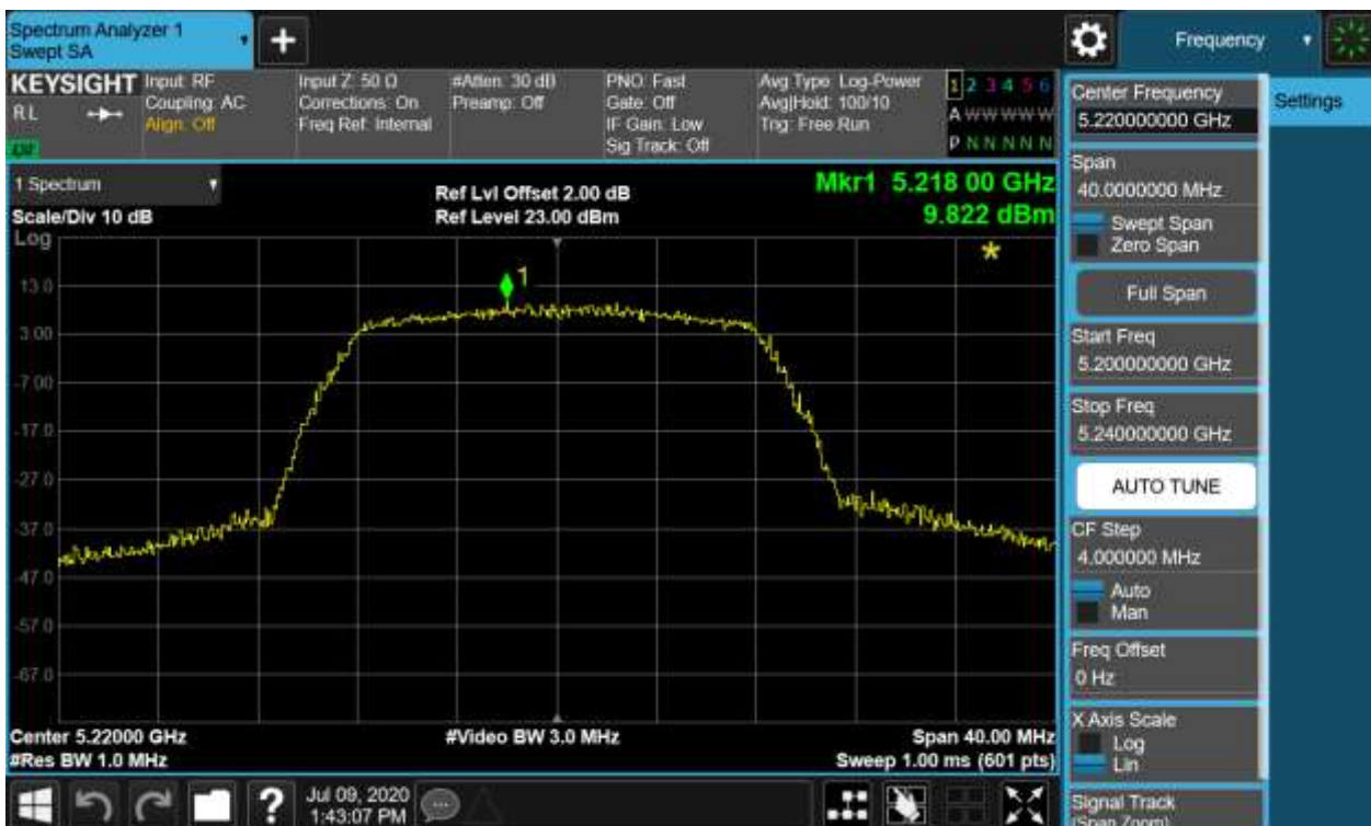
Figure 44: Power Spectral Density, 802.11a, 5220MHz
