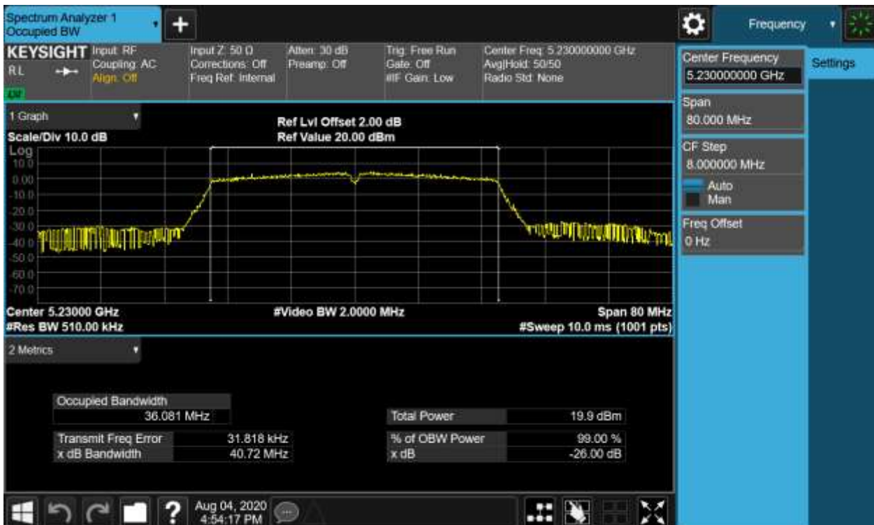
Figure 11: 26dB Bandwidth and 99% Bandwidth, 802.11n(HT40), 5230MHz
