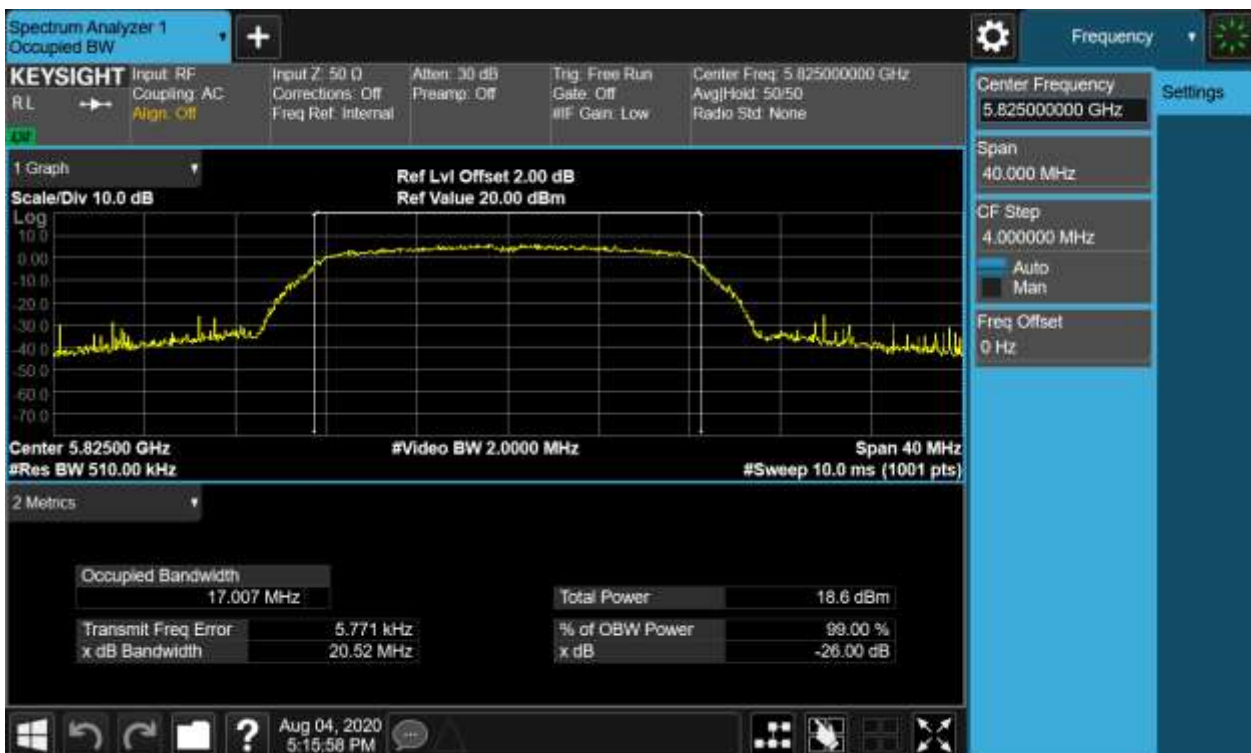
Figure 17: 26dB Bandwidth and 99% Bandwidth, 802.11a, 5825MHz
