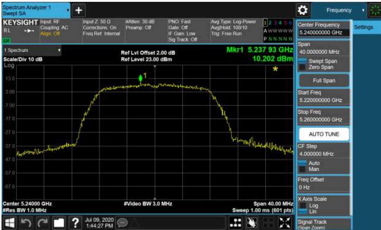
Figure 45: Power Spectral Density, 802.11a, 5240MHz
