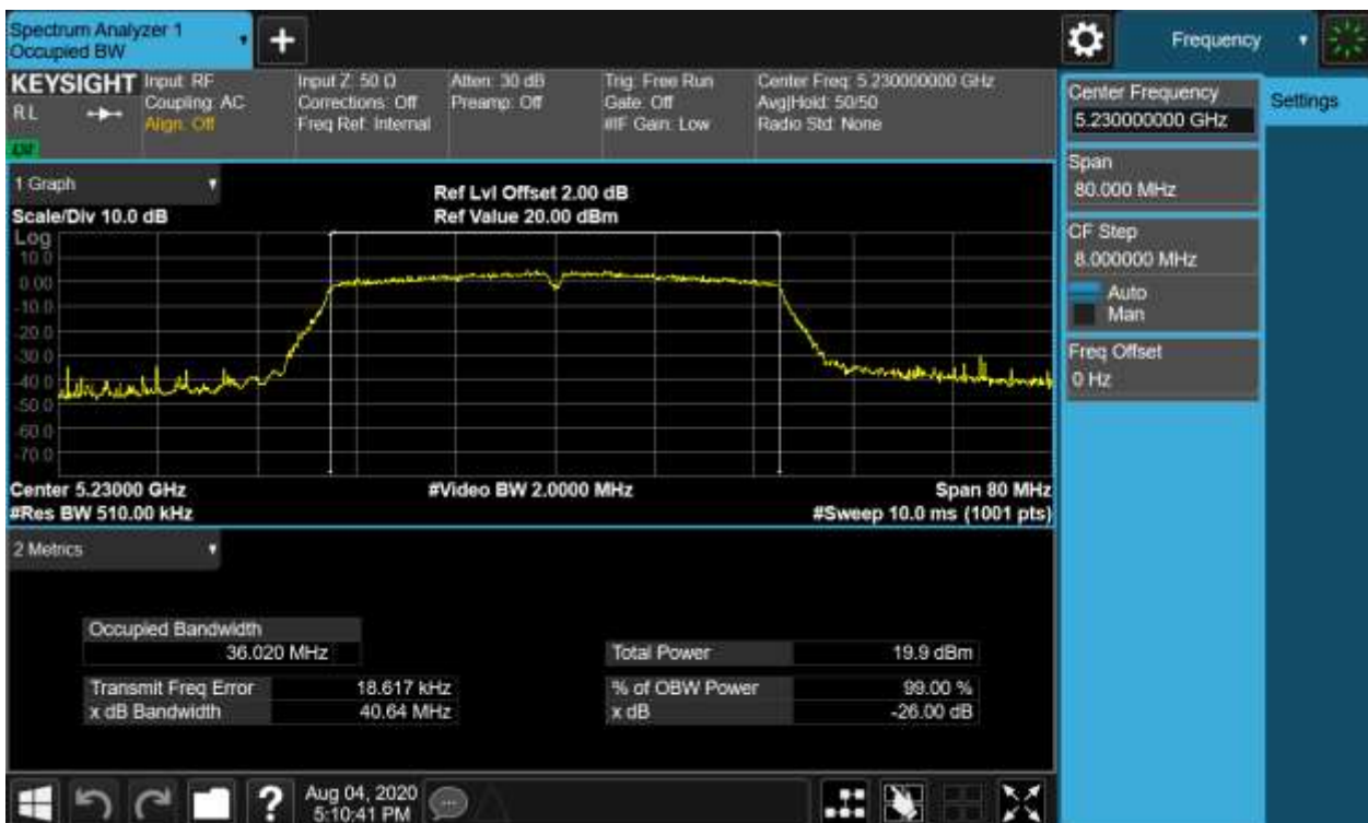
Figure 13: 26dB Bandwidth and 99% Bandwidth, 802.11ac(VHT40), 5230MHz
