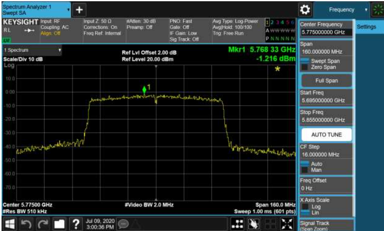
Figure 70: Power Spectral Density, 802.11ac(VHT80), 5775MHz
