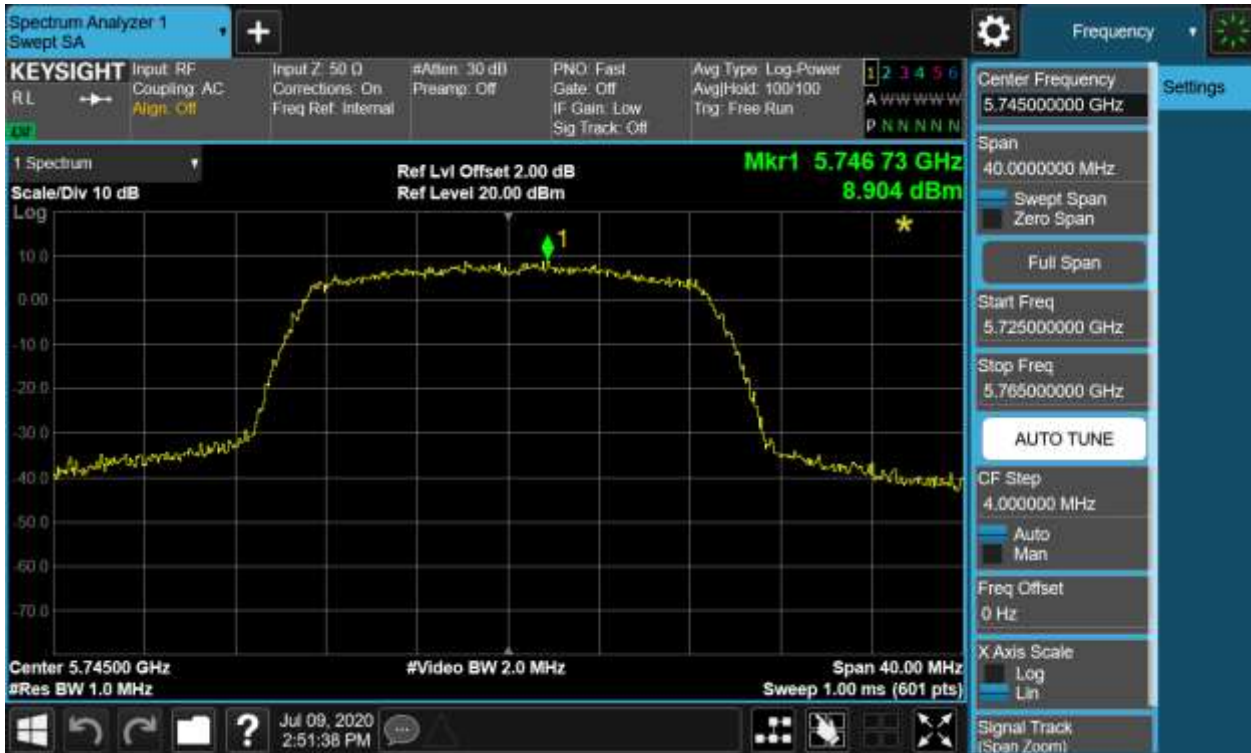
Figure 63: Power Spectral Density, 802.11ac(VHT20), 5745MHz
