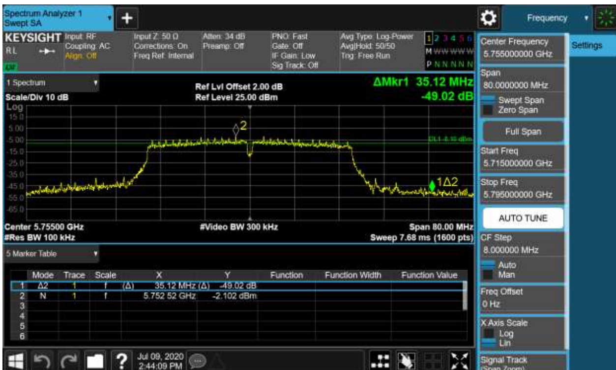
Figure 38: 6dB Bandwidth, 802.11n(HT40), 5755MHz
