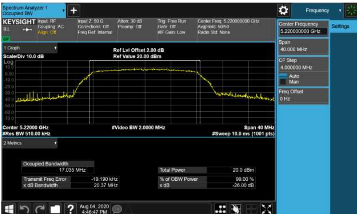
Figure 2: 26dB Bandwidth and 99% Bandwidth, 802.11a, 5220MHz
