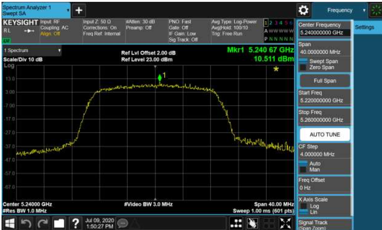
Figure 51: Power Spectral Density, 802.11ac(VHT20), 5240MHz
