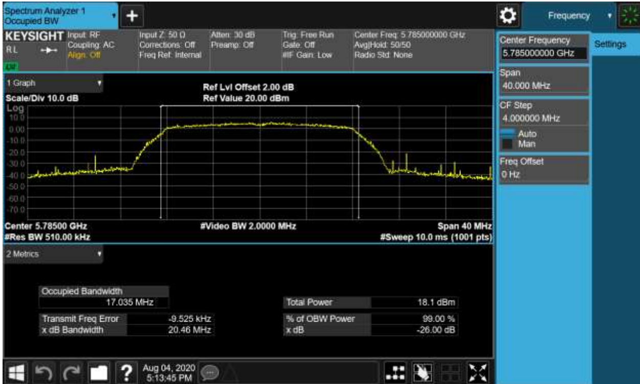
Figure 16: 26dB Bandwidth and 99% Bandwidth, 802.11a, 5785MHz
