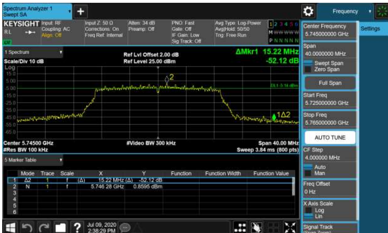
Figure 32: 6dB Bandwidth, 802.11n(HT20), 5745MHz
