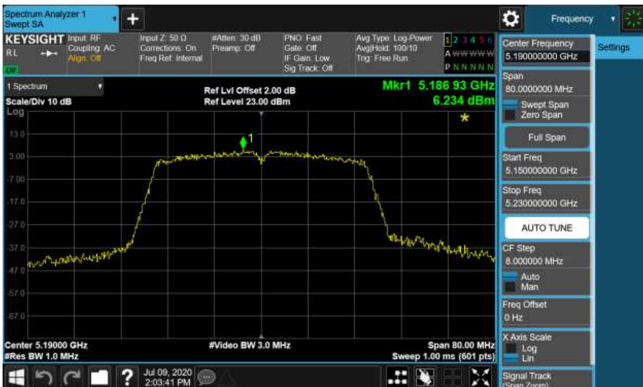
Figure 52: Power Spectral Density, 802.11n(HT40), 5190MHz
