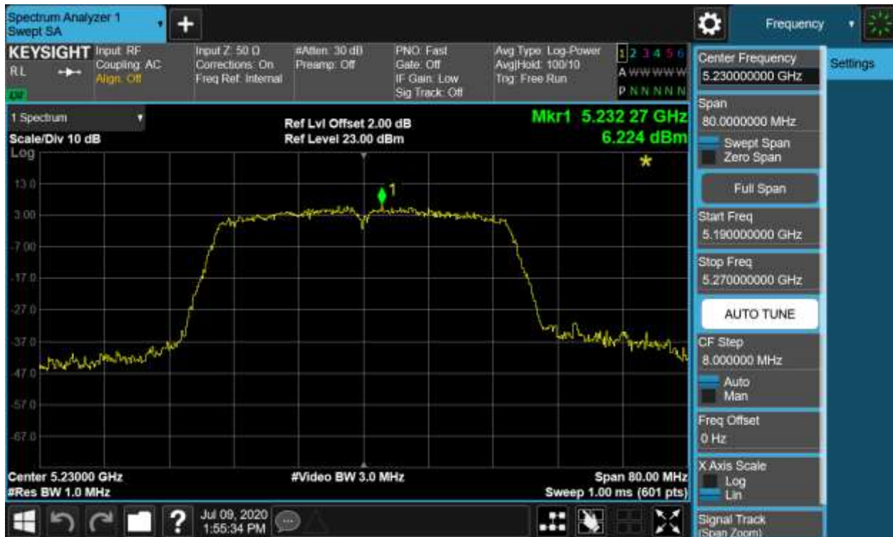
Figure 55: Power Spectral Density, 802.11ac(VHT40), 5230MHz
