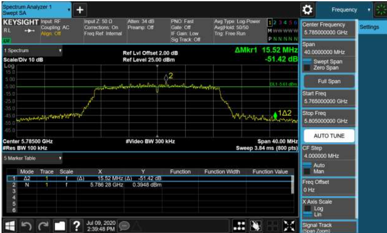
Figure 33: 6dB Bandwidth, 802.11n(HT20), 5785MHz
