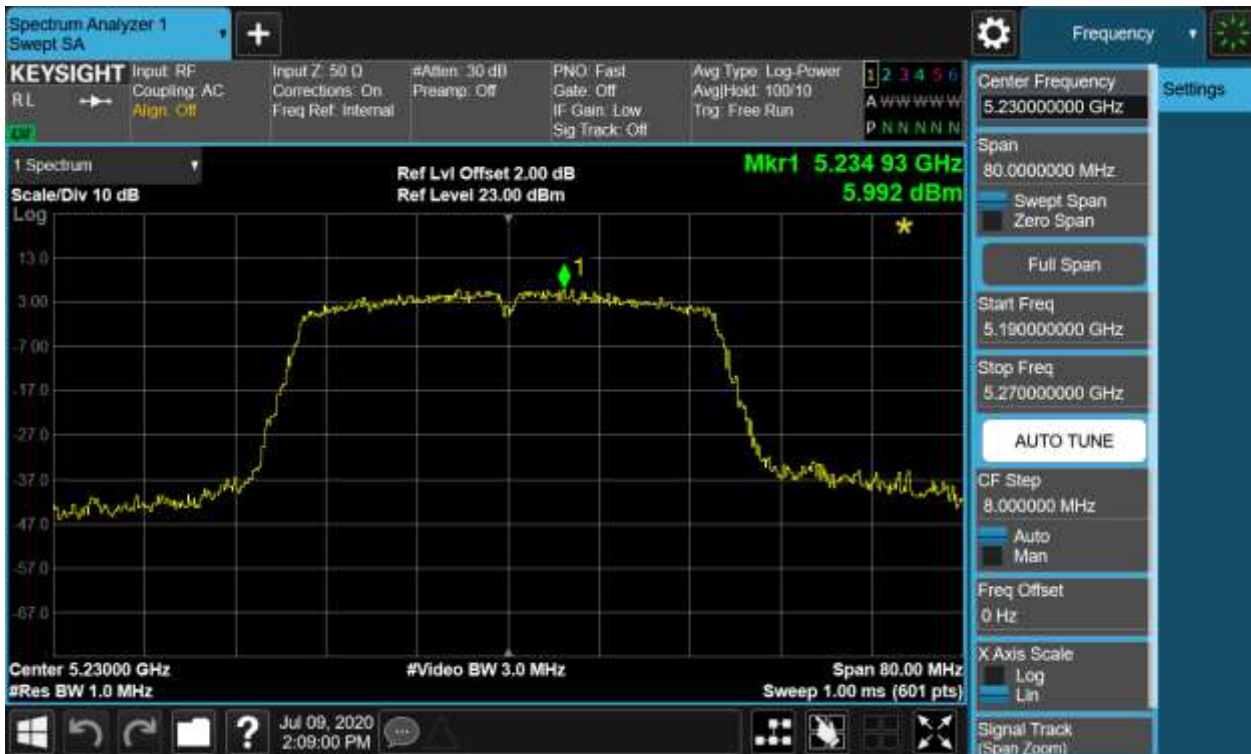
Figure 53: Power Spectral Density, 802.11n(HT40), 5230MHz
