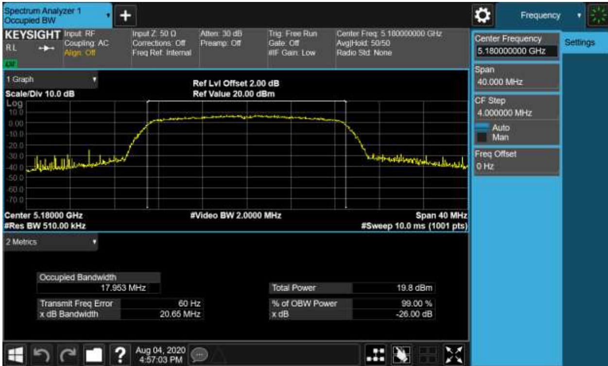
Figure 7: 26dB Bandwidth and 99% Bandwidth, 802.11ac(VHT20), 5180MHz
