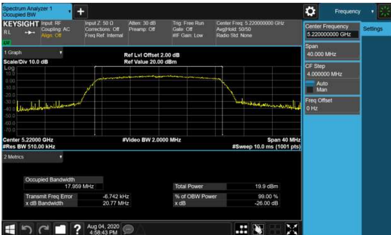
Figure 8: 26dB Bandwidth and 99% Bandwidth, 802.11ac(VHT20), 5220MHz
