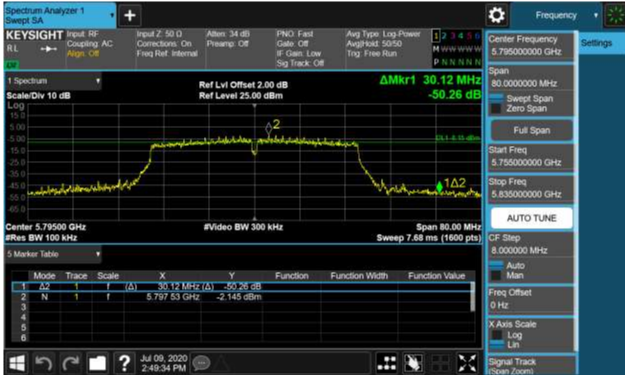
Figure 39: 6dB Bandwidth, 802.11n(HT40), 5795MHz
