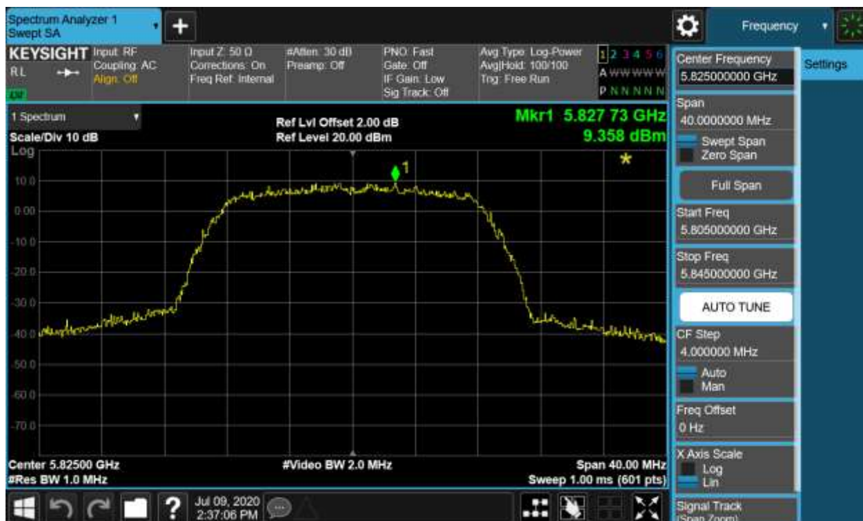
Figure 59: Power Spectral Density, 802.11a, 5825MHz
