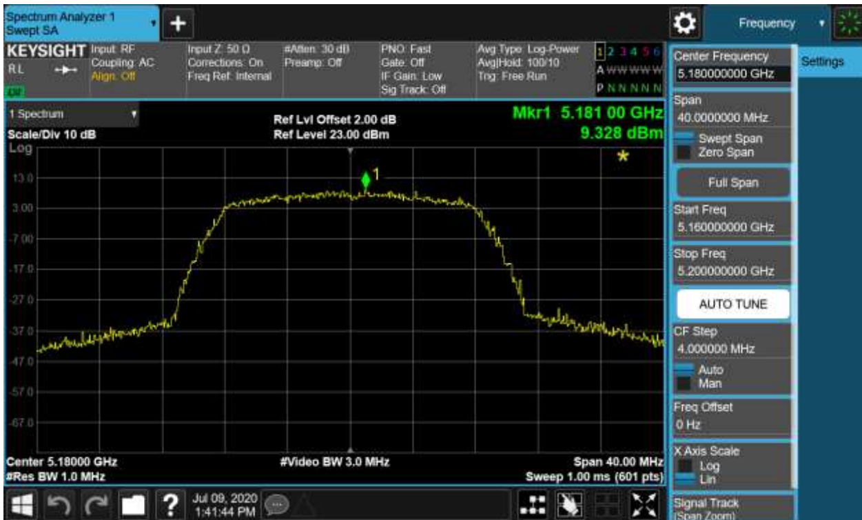
Figure 43: Power Spectral Density, 802.11a, 5180MHz
