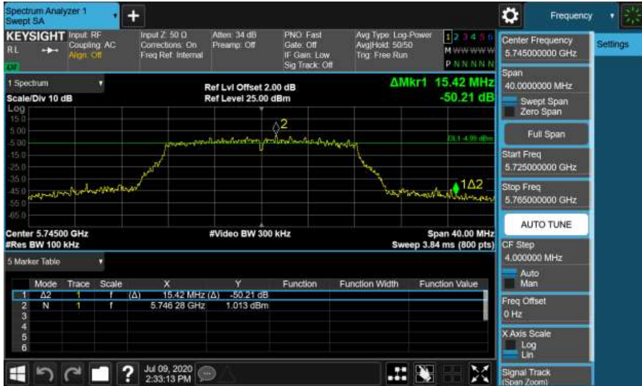
Figure 29: 6dB Bandwidth, 802.11a, 5745MHz
