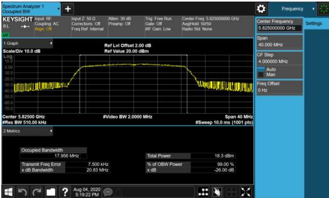
Figure 20: 26dB Bandwidth and 99% Bandwidth, 802.11n(HT20), 5825MHz
