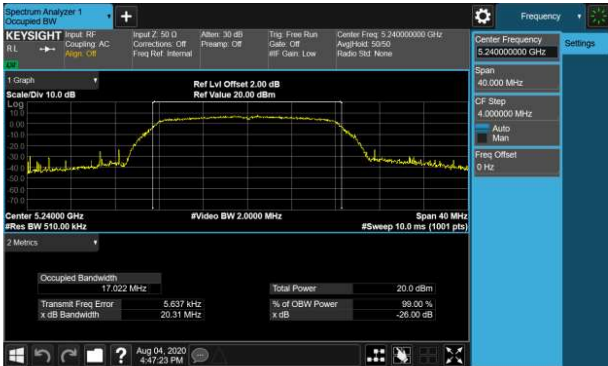
Figure 3: 26dB Bandwidth and 99% Bandwidth, 802.11a, 5240MHz
