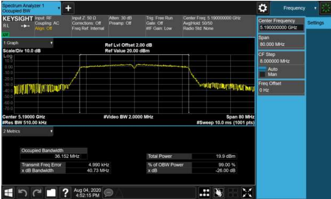
Figure 10: 26dB Bandwidth and 99% Bandwidth, 802.11n(HT40), 5190MHz
