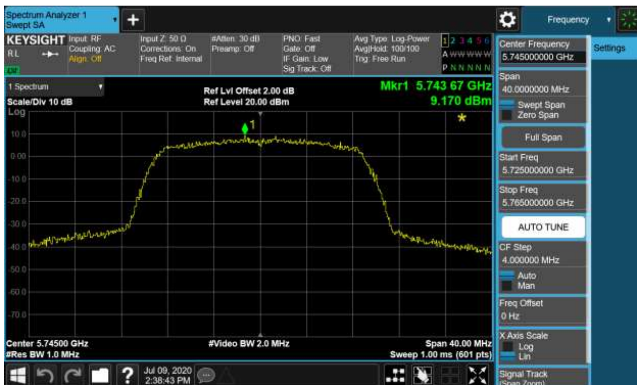
Figure 60: Power Spectral Density, 802.11n(HT20), 5745MHz
