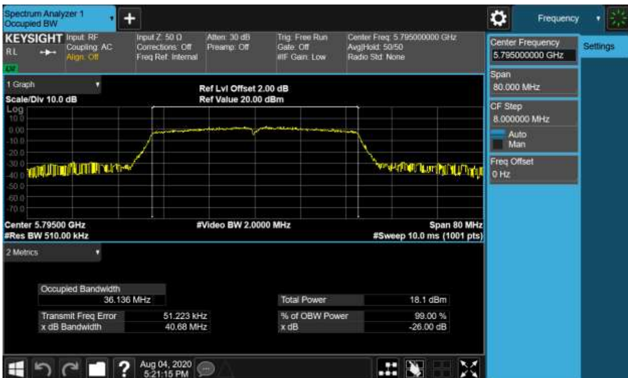
Figure 25: 26dB Bandwidth and 99% Bandwidth, 802.11n(HT40), 5795MHz
