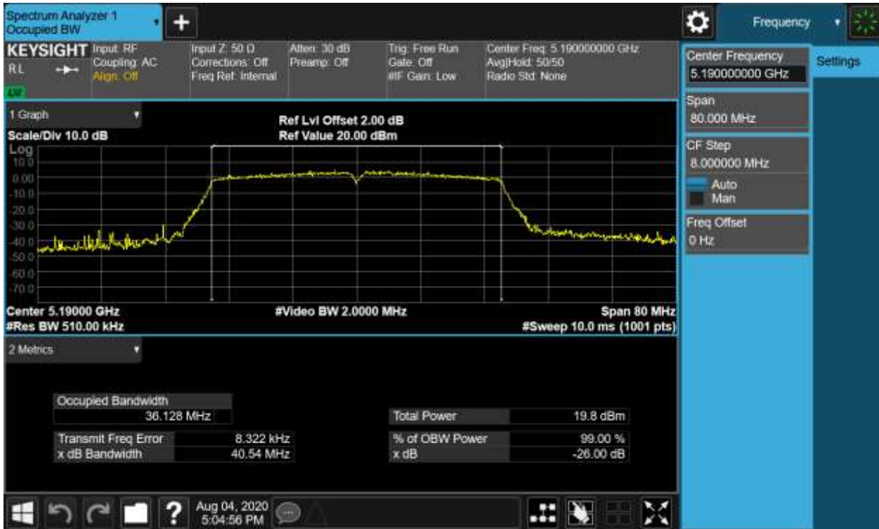
Figure 12: 26dB Bandwidth and 99% Bandwidth, 802.11ac(VHT40), 5190MHz
