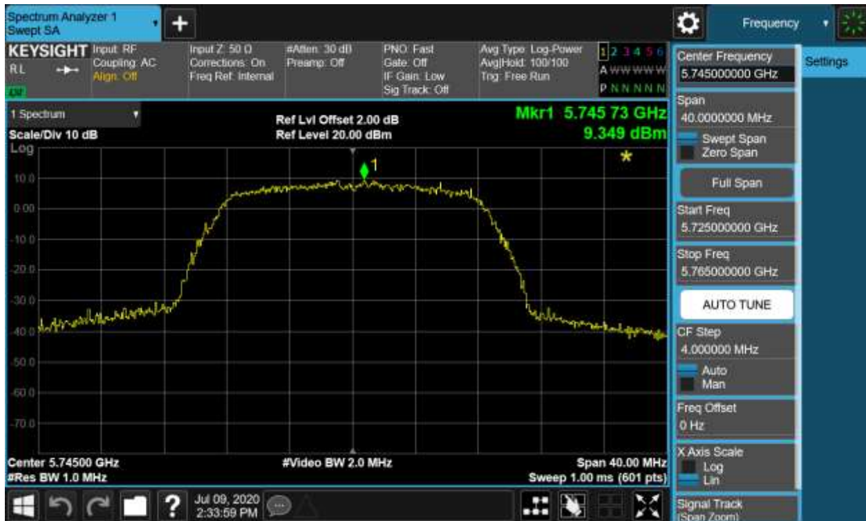
Figure 57: Power Spectral Density, 802.11a, 5745MHz
