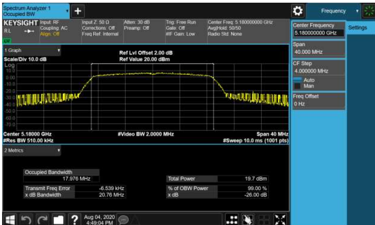
Figure 4: 26dB Bandwidth and 99% Bandwidth, 802.11n(HT20), 5180MHz
