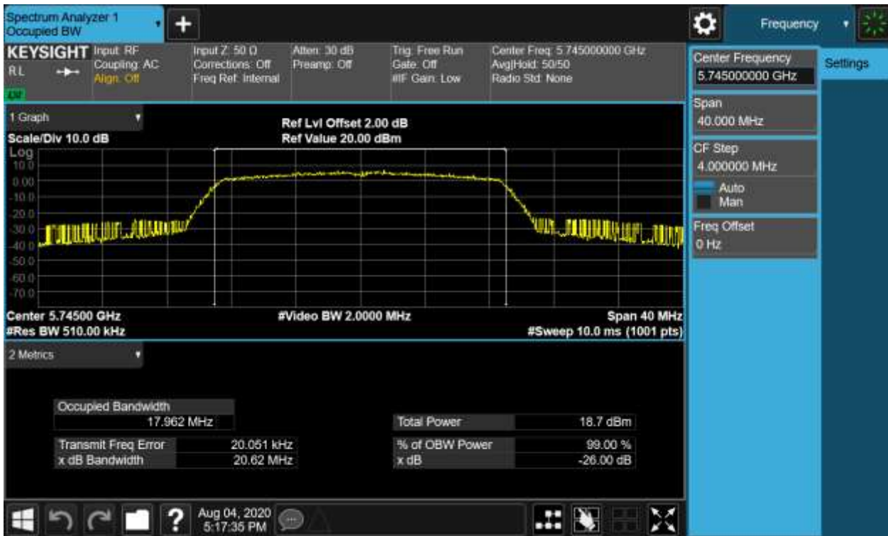
Figure 18: 26dB Bandwidth and 99% Bandwidth, 802.11n(HT20), 5745MHz
