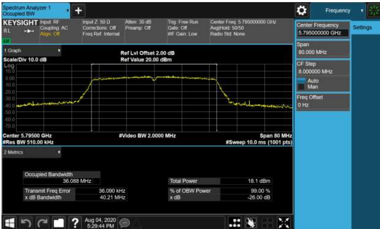
Figure 27: 26dB Bandwidth and 99% Bandwidth, 802.11ac(VHT40), 5785MHz
