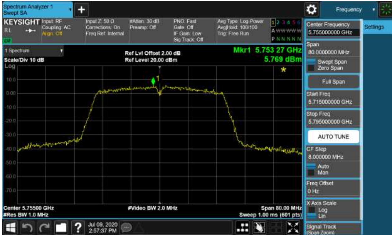
Figure 68: Power Spectral Density, 802.11ac(VHT40), 5755MHz
