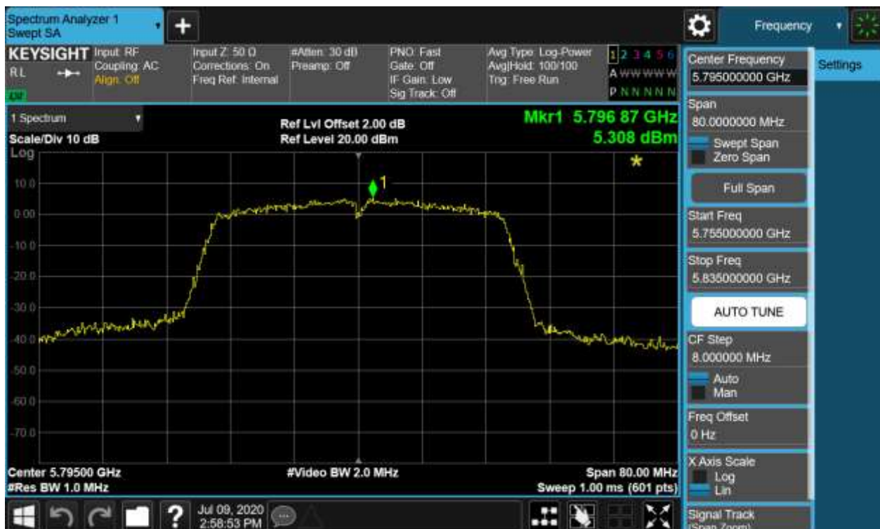
Figure 69: Power Spectral Density, 802.11ac(VHT40), 5785MHz
