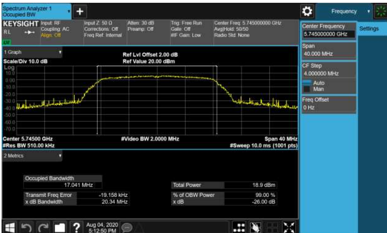
Figure 15: 26dB Bandwidth and 99% Bandwidth, 802.11a, 5745MHz
