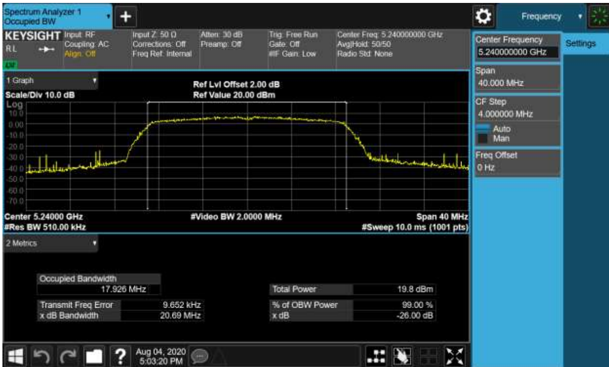
Figure 9: 26dB Bandwidth and 99% Bandwidth, 802.11ac(VHT20), 5240MHz
