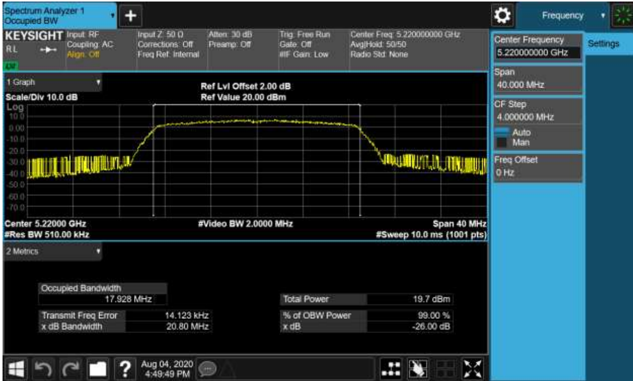
Figure 5: 26dB Bandwidth and 99% Bandwidth, 802.11n(HT20), 5220MHz
