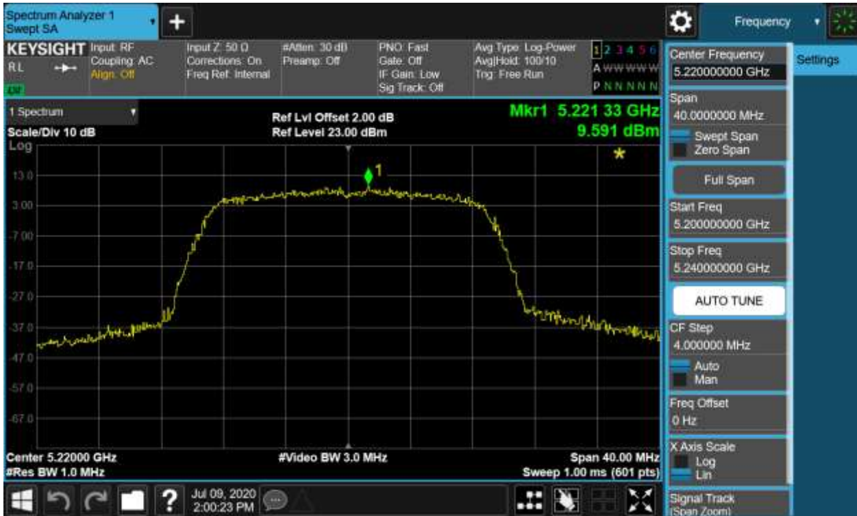
Figure 47: Power Spectral Density, 802.11n(HT20), 5220MHz
