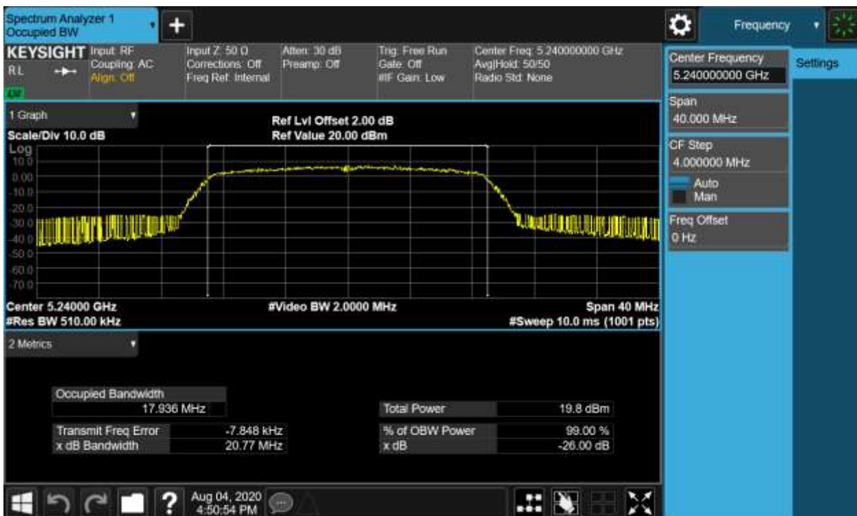
Figure 6: 26dB Bandwidth and 99% Bandwidth, 802.11n(HT20), 5240MHz
