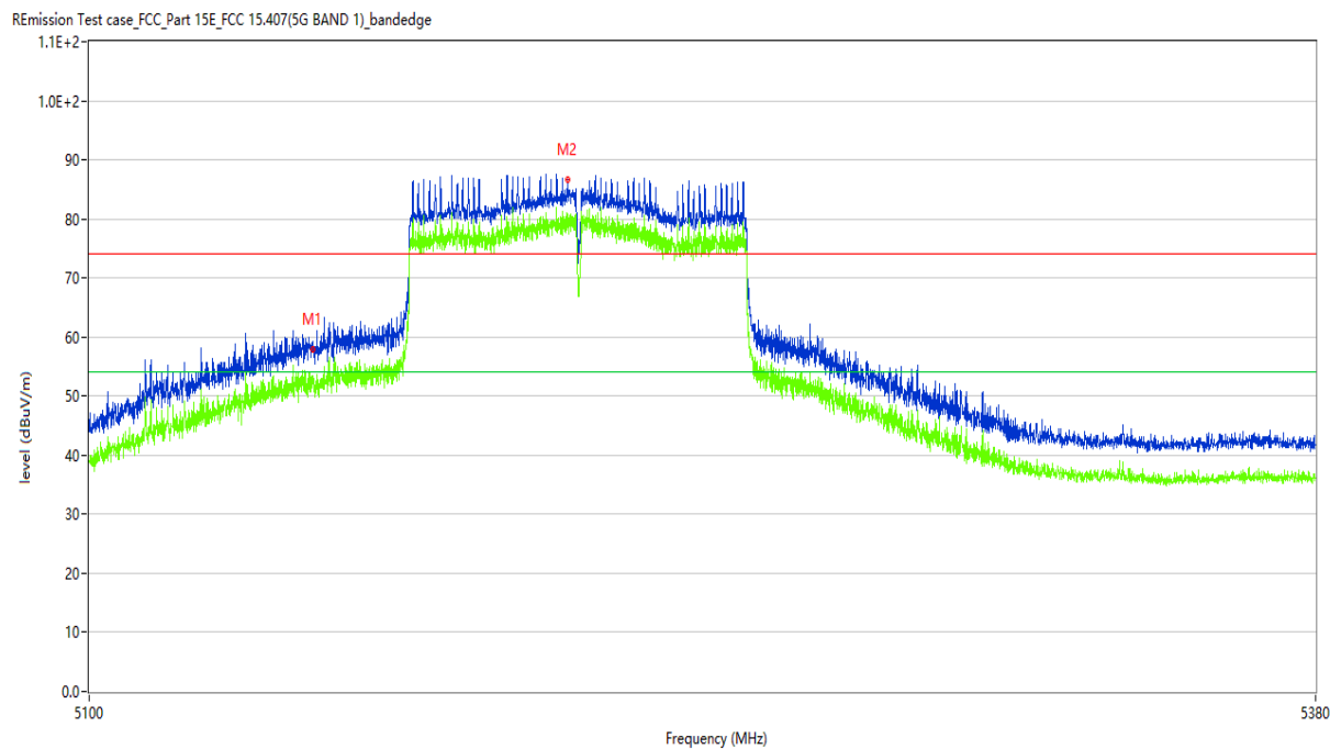
Figure 138: Band Edge (Restricted-band band-edge), 802.11ac(VHT80), 5210MHz
