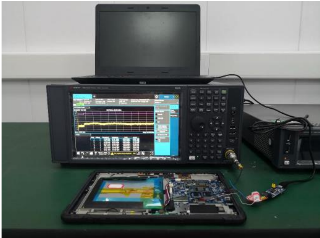
Conducted RF test at Antenna Port
